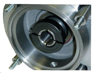
lems. With a C Face connection the motor shaft typically slides into a hollow quill in the brake or clutch brake. A key and keyway are used to prevent rotation between the shaft and quill. This means that the fit must be loose enough for simple installation or removal.
