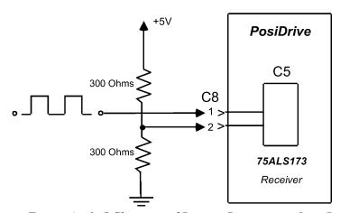
Figure A - 1: RChematic of Biasing Resistors on Line Receiver
