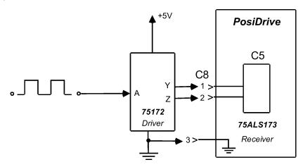
Figure A - 2: RChematic of Line Driver to Line Receiver
