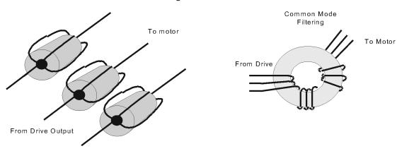
Common mode currents occur from noise spikes created by the PWM switching frequency of the *PosiDrive RC*. The use of a ferrite or iron-powder core toroid places common mode impedance in the line between the motor and the *PosiDrive RC*. The use of a common mode choke on the motor leads may increase signal integrity of encoder outputs and associated I/O signals. A list of toroidal and ferrite cores that can be used to make common mode chokes is found in the following tables.
