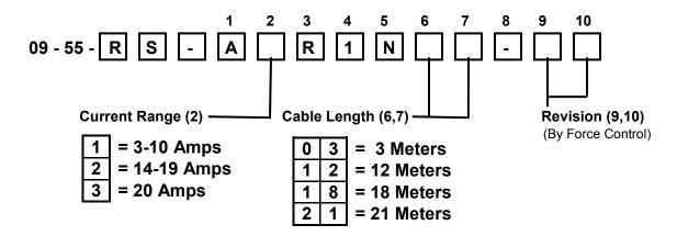
**NOTE:** Use the Model Number above to order a correct Set of Cables. A complete set of Cables includes (1) Servomotor Cable and (1) Resolver Cable as shown in Figure 2.2 below. Cables can only be ordered in 3 meter increments (i.e. 3m, 6m, 9m, 12m, etc).
