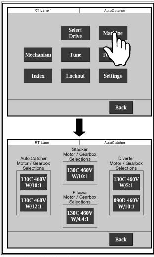
Figure 6.4 - Machine Screen
