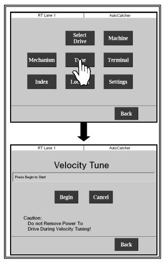
Figure 6.12 -- Velocity Tune Screen
