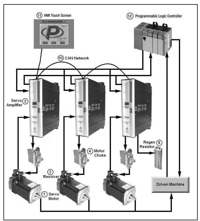
Figure 1.1 – PosiDrive Servo System Diagram
