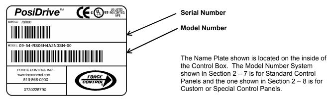
Figure 2.3 - Control Panel Name Plate
