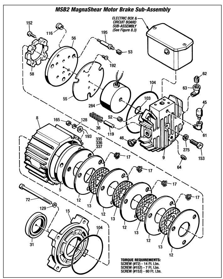
Figure 8.2 Repair Parts - MSB2 MagnaShear Motor Brake
