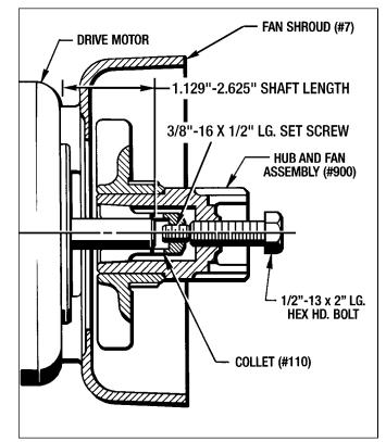
Figure 7.4 - Removing Hub (#2) and Collet (#110)
