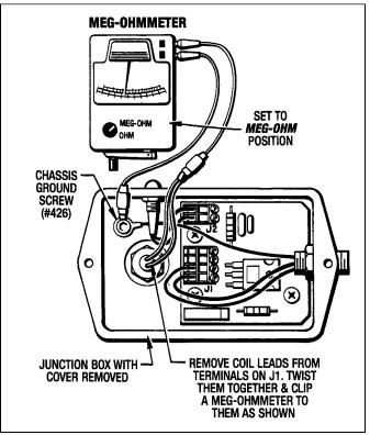
Figure 6.2- Coil Current Leakage Testing
