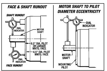
Figure 3.1 - Verifying Motor Specifications
