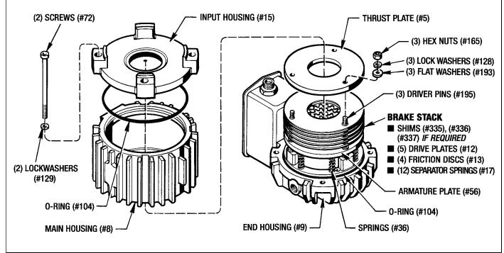
Figure 7.2 - Replacing the Brake Stack
