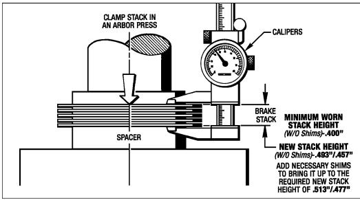
Figure 7.1 - Measuring Stack Height
