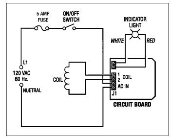
Figure 5.1 - Test Set-Up Electrical Schematic
