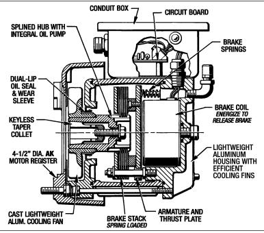
Figure 1.2 - MagnaShear MSB2 Motor Brake Cross Section
