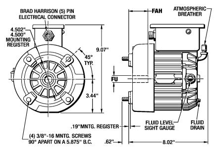
Std. Motor Shaft Tolerances: .625" Dia & .875"Dia. (+.0000" -.0005") Std. Motor Register Tolerances: 4.500"Dia. (+.000" -.003")
