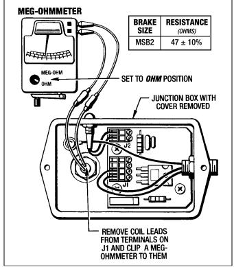
Figure 6.1 - Coil Resistance Testing
