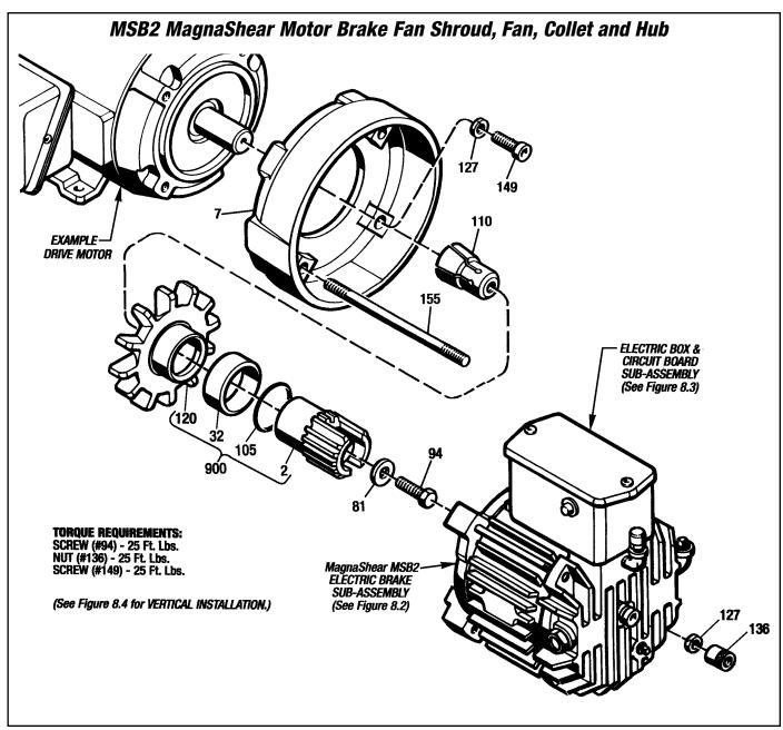
Figure 8.1 - MSB2 MagnaShear Motor Brake - Fan Shroud, Fan, Collet and Hub
