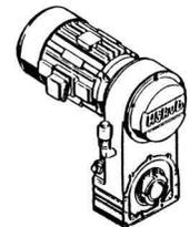
1. First, remove the Chain Access Cover (#271) by removing (6) screws (#63) from the Transfer Case Housing (#270). Remove Gasket (#77).
