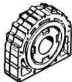
1. Install O-Rings (#39) and Liners (#42) into Piston Retainers and Piston Housings. Lubricate O-Rings before installation. (See Figure 9.10)
