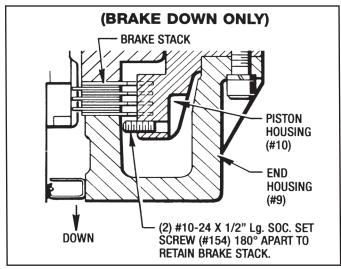
Figure 7 - Brake Stack Retaining Screws (Brake Down)
