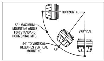
Figure 12 - Mounting Angle (Brake Down)
