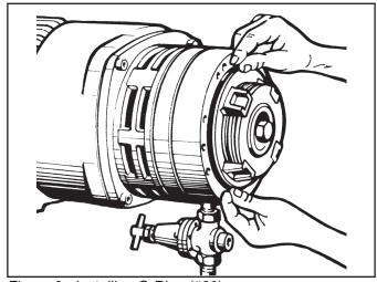
Figure 8 - Installing O-Ring (#30)
