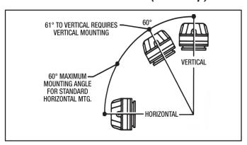
Figure 10 - Mounting Angle (Brake Up)
