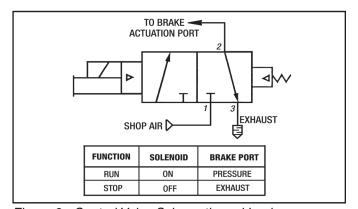
Figure 9 - Control Valve Schematic and Logic
