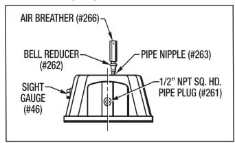
Figure 11 - Air Breather Installation
