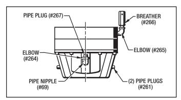
Figure 13 - Air Breather Installation (Brake Down)
