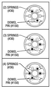
Figure 5 - Spring Placement Install the radius side
