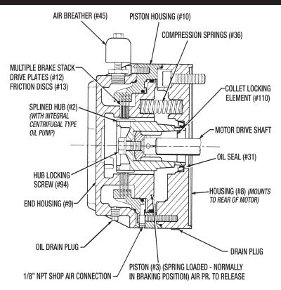
Figure 1 - Unit Description and Operation
