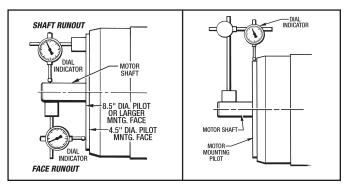
Figure 2 - Verifying Motor Specifications
