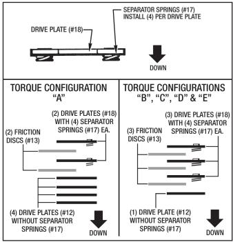
Figure 6 - Installing Separator Springs on Vertical Units
