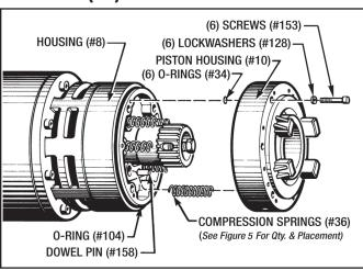
Figure 4 - Mounting Piston Housing Assembly
