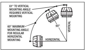
Figure 3.12 MOUNTING ANGLE (Brake Up)
