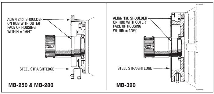
Figure 3.3 HUB ALIGNMENT - STEP 2
