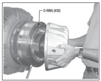
Figure 3.9 INSTALLING END HOUSING
