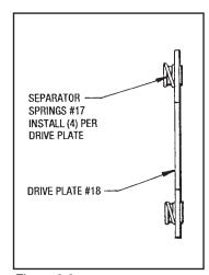
Figure 3.8 SEPARATOR SPRINGS
