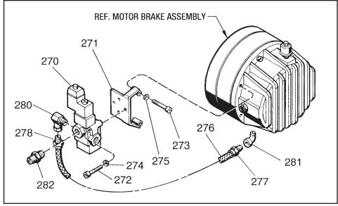
Figure 8.1 CONTROL VALVE MOUNTING KIT
