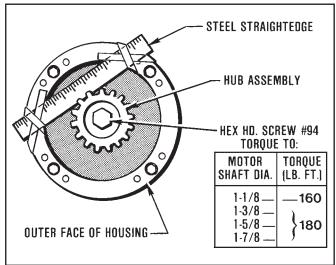
Figure 3.2 HUB ALIGNMENT - STEP 1
