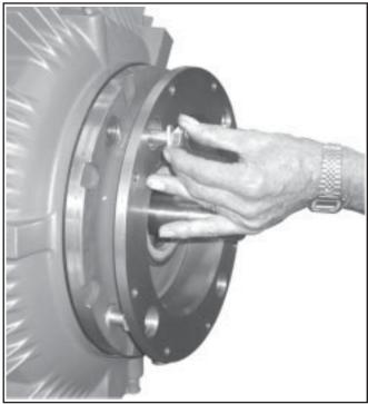
Figure 3.1 INSTALLING HOUSING (#8 ) TO MOTOR FLANGE
