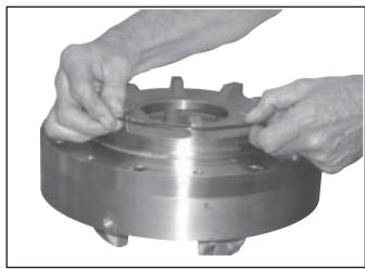
Figure 3.5 INSTALLING O-RING (#33)
