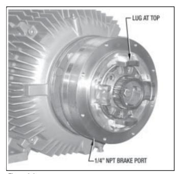
Figure 3.6 CORRECT POSITION OF PISTON HOUSING ASSEMBLY
