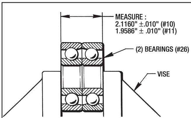
Figure 9.1 - Measuring Thickness of Bearings (#26)
