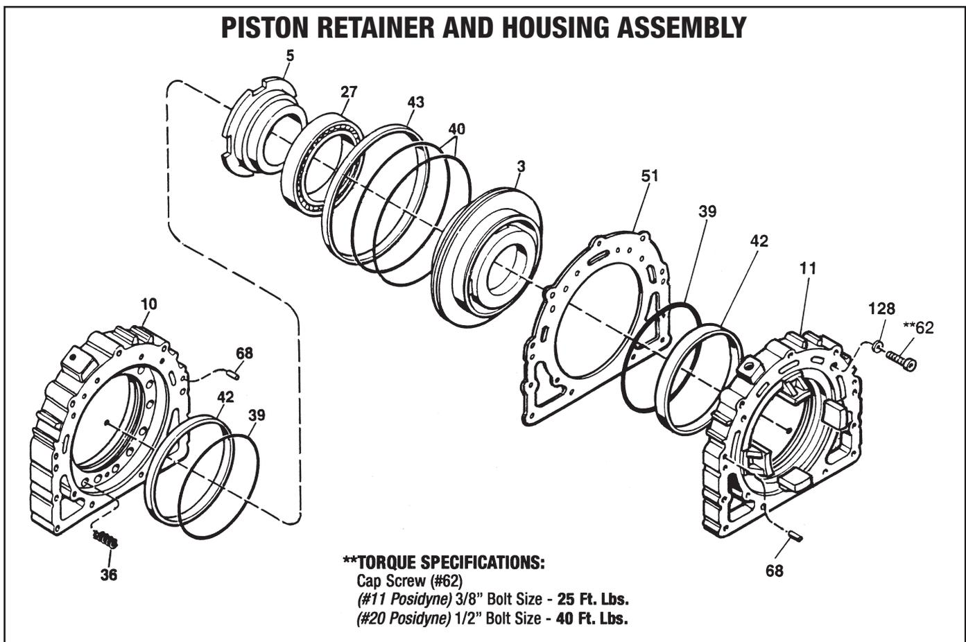
Figure 10.4 - Piston Retainer and Housing Assembly
