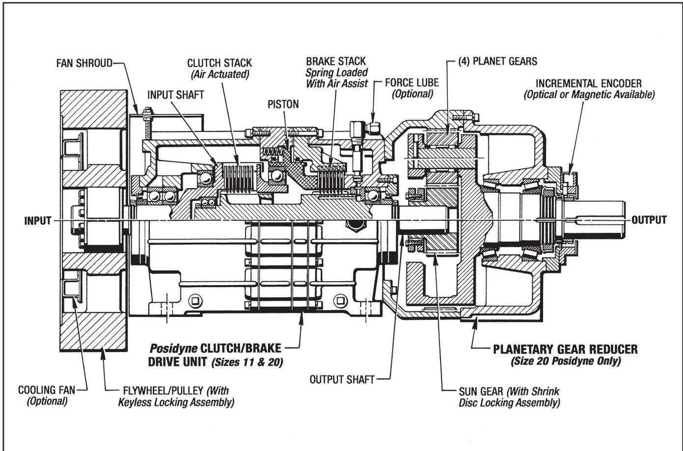
Figure 1.2 - Posidyne Indexing Clutch/Brake Drive
