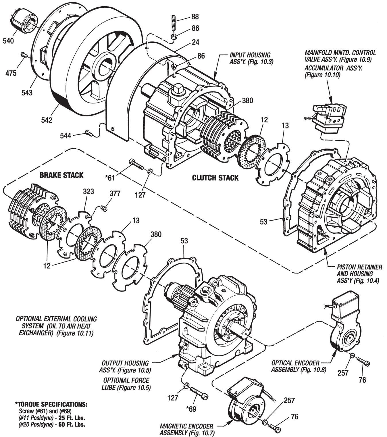
Figure 10.1 - #11 and #20 Posidyne Indexing Drive (Without Planetary Gear Reducer)
