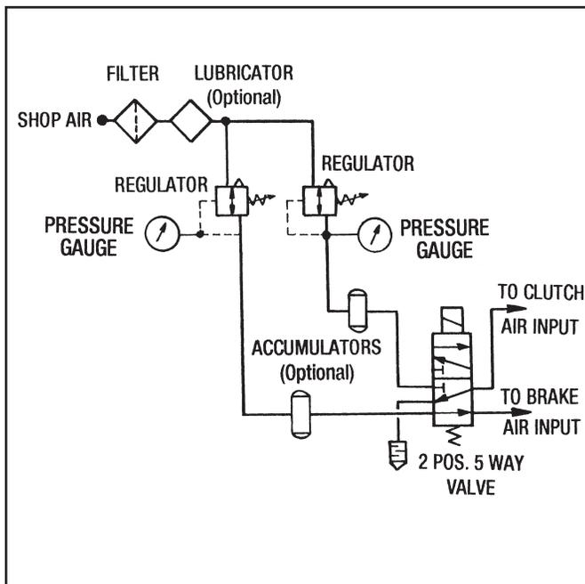
Figure 3.3 - Pneumatic Schematic
