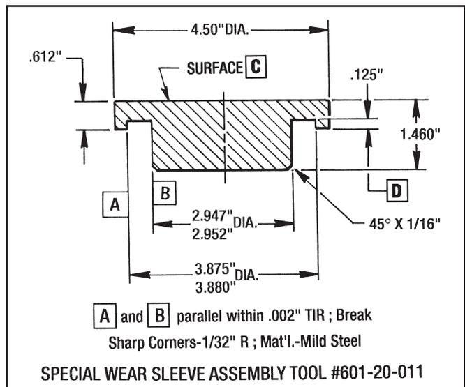
Figure 9.7 - Wear Sleeve Assembly Tool for #20 Posidyne
