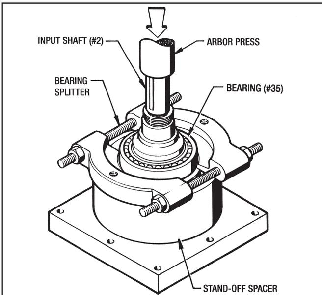
Figure 7.5 - Removing Bearing from the Input Shaft
