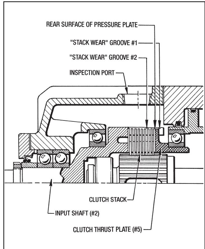
Figure 6.2 - Checking Brake and Clutch Stacks for Wear
