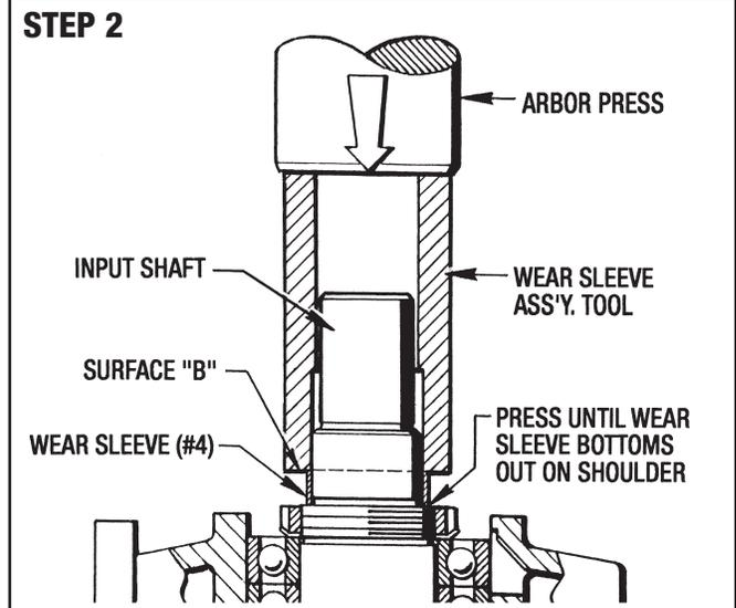
Figure 9.6 - Installing Wear Sleeve (#4) on #11 Posidyne
