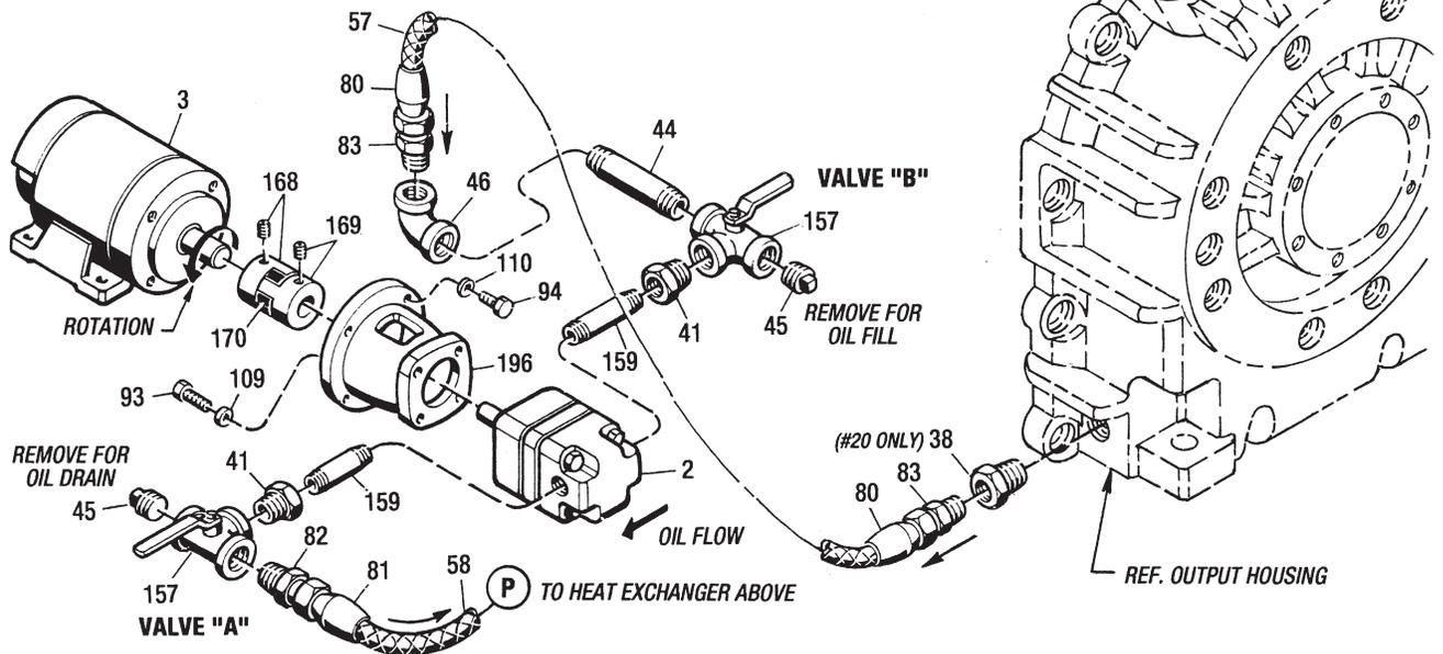
Figure 10.11 - External Cooling System
