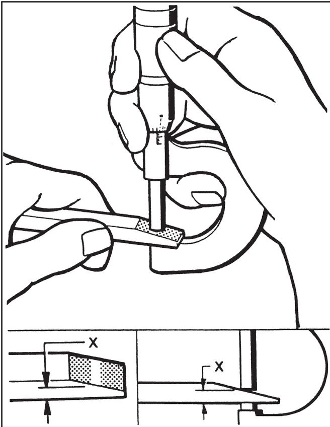
Figure 9.12 - Measuring Piston Stroke
