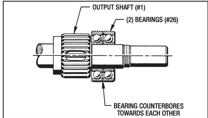
Figure 9.2 - Installing Bearings (#26) (Without Force Lube)
