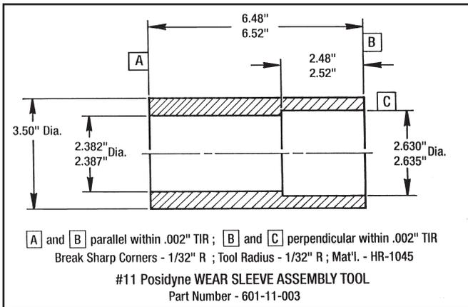
Figure 9.5 - Wear Sleeve Assembly Tool for #11 Posidyne
