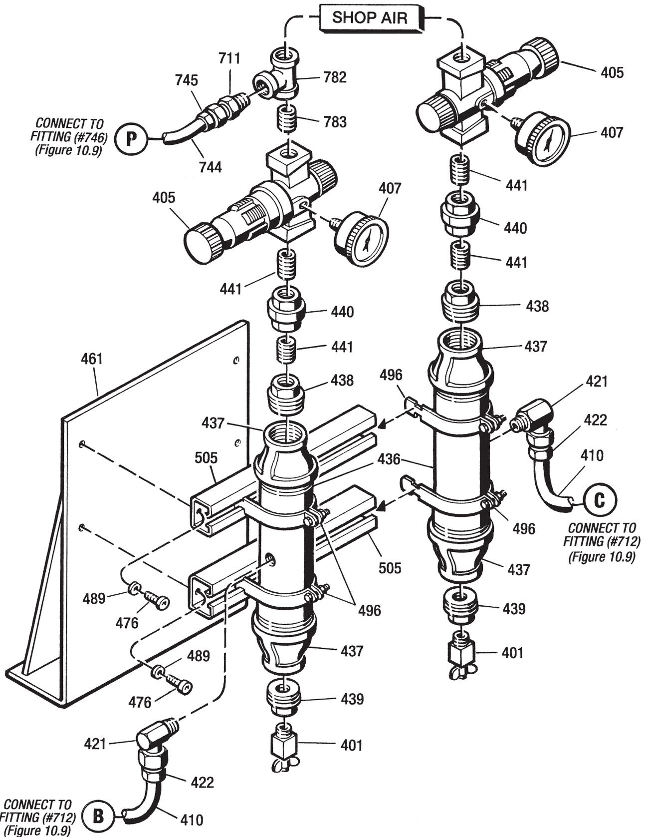
Figure 10.10 - Pneumatic Accumulator Assembly
