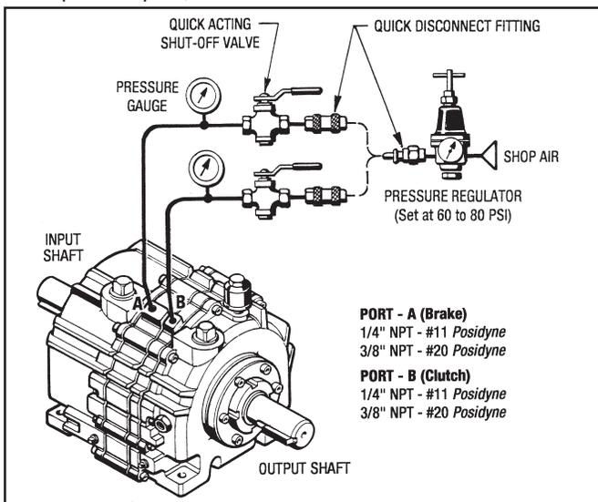
Figure 5.1 - Pneumatic Testing Set-Up for Operational Check
