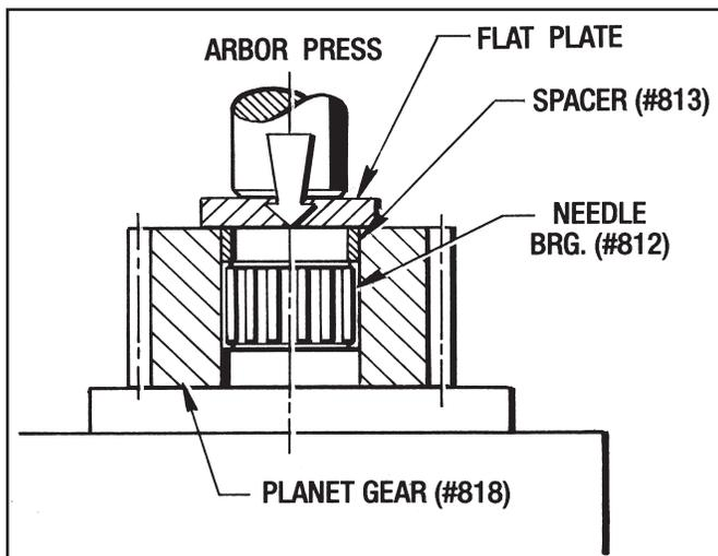
Figure 9.21 - Installing Needle Bearings (#812)
