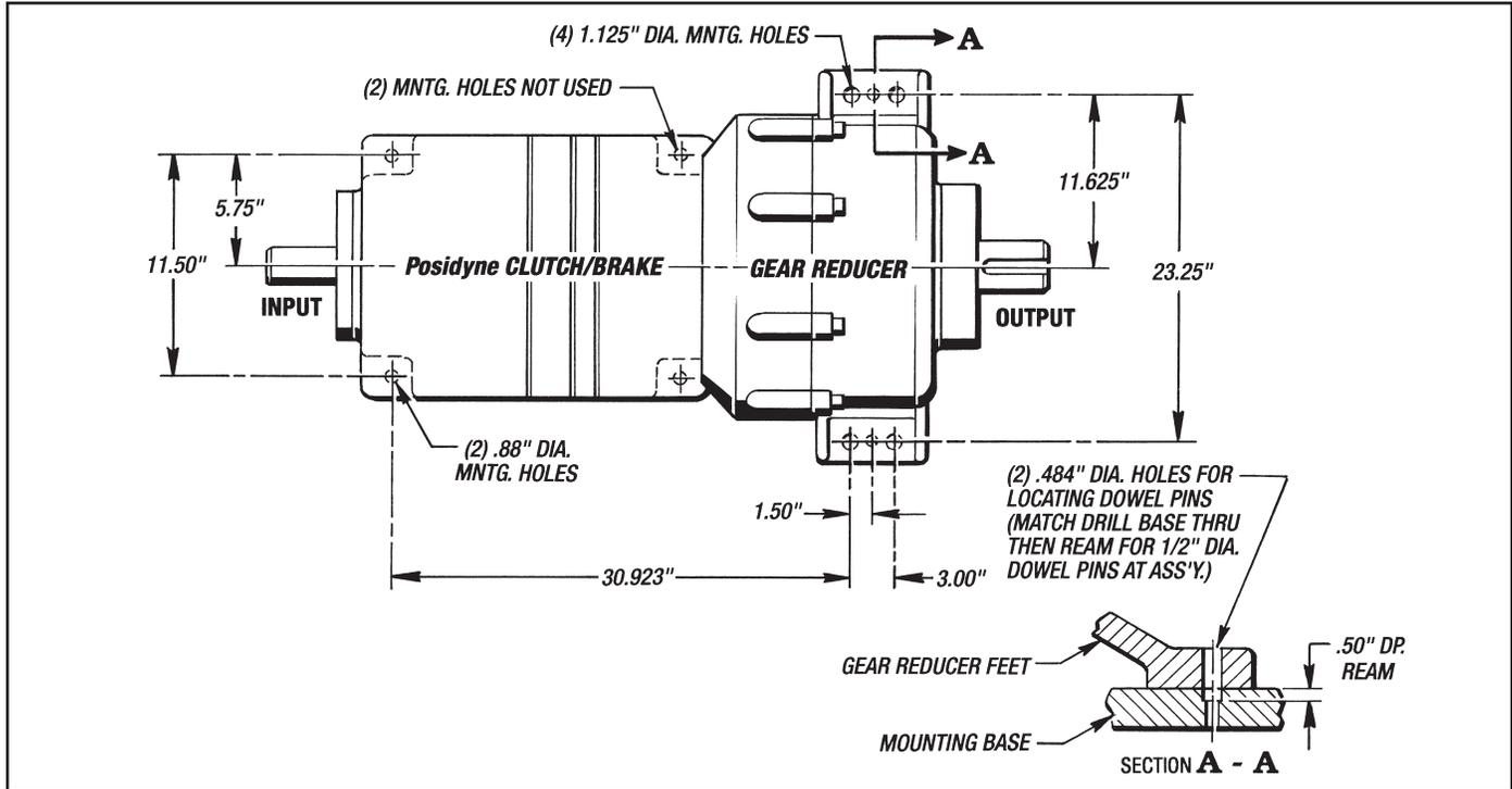
Figure 3.2 - Mounting Hole Layout and Installing Mounting Dowel Pins
