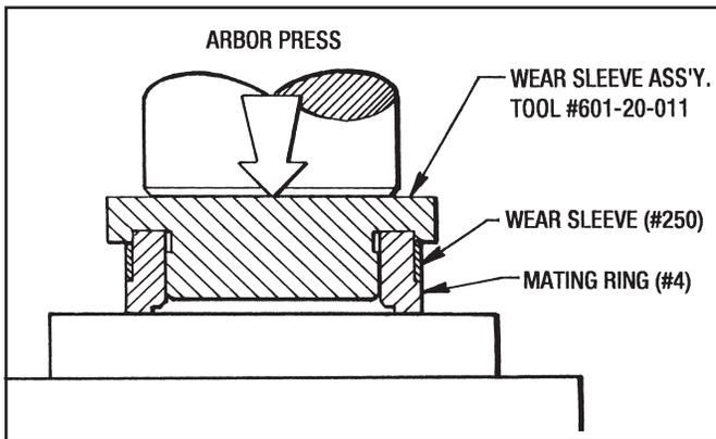
Figure 9.8 - (Step 2) Installing Wear Sleeve (#250) on Mating Ring (#4) for #20 Posidyne
