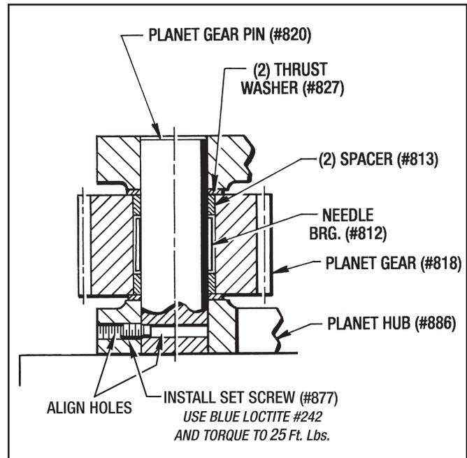
Figure 9.22 - Installing Planet Gears
