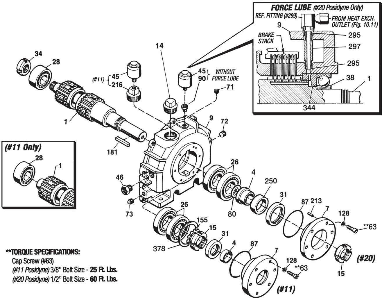
Figure 10.5 - Output Housing Assembly
