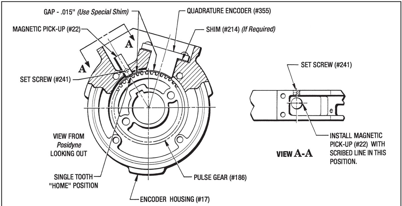
Figure 9.17 - Position Sensors Installation
