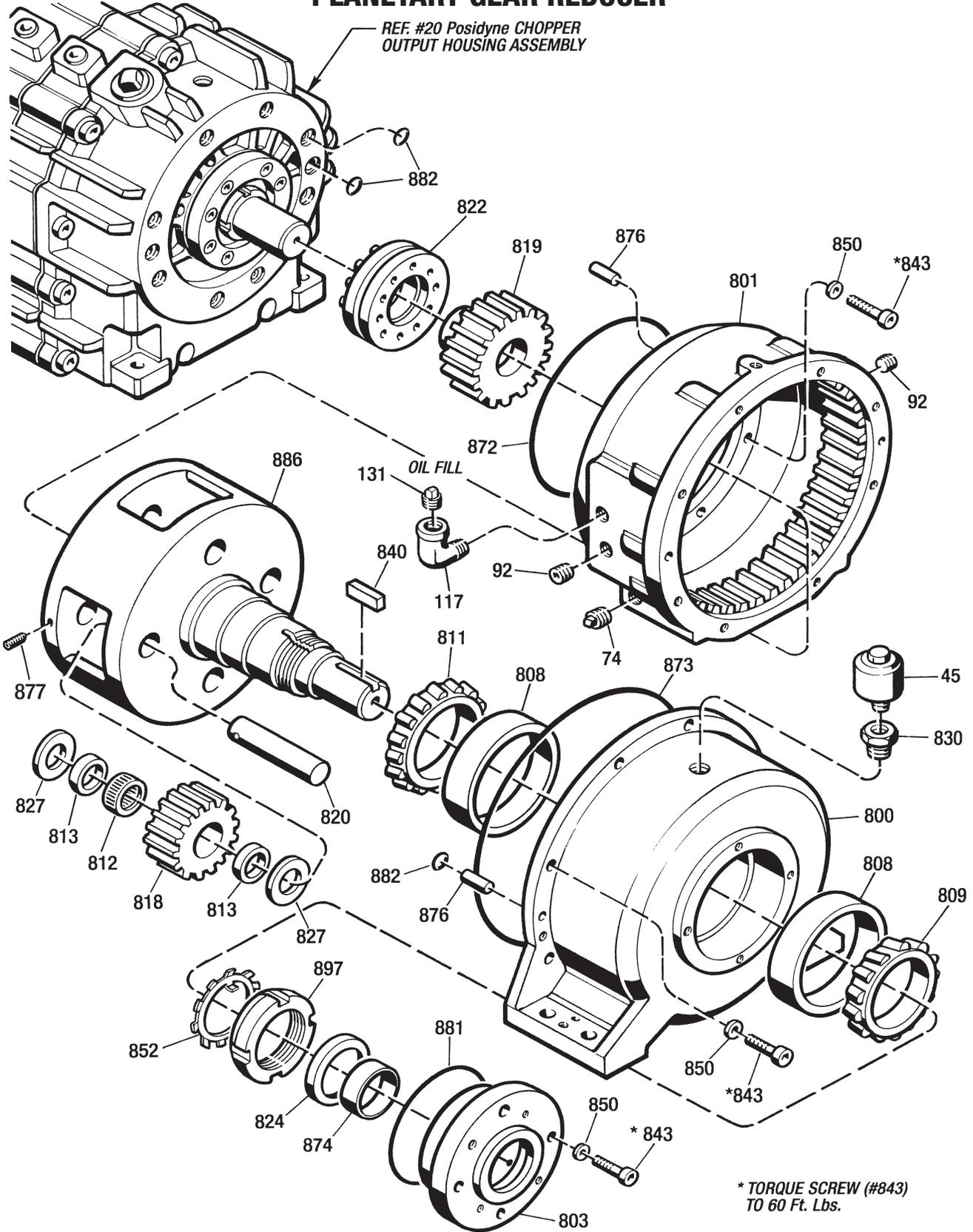
Figure 10.6 - Planetary Gear Reducer
