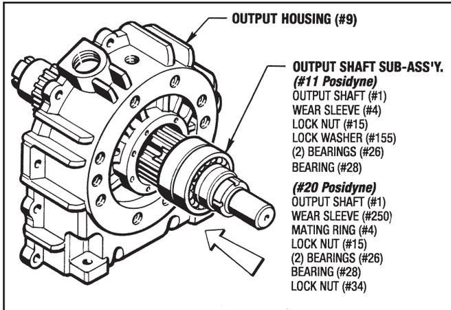
Figure 9.3 - Installing Output Shaft Sub-Assembly
