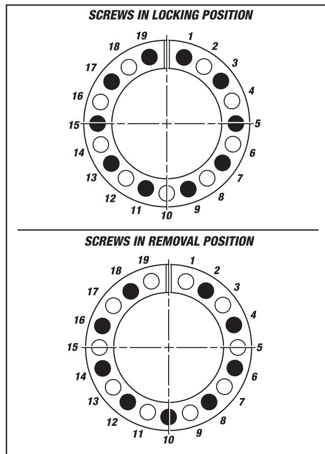
Figure 7.1 - Flywheel Locking Assembly Removal
