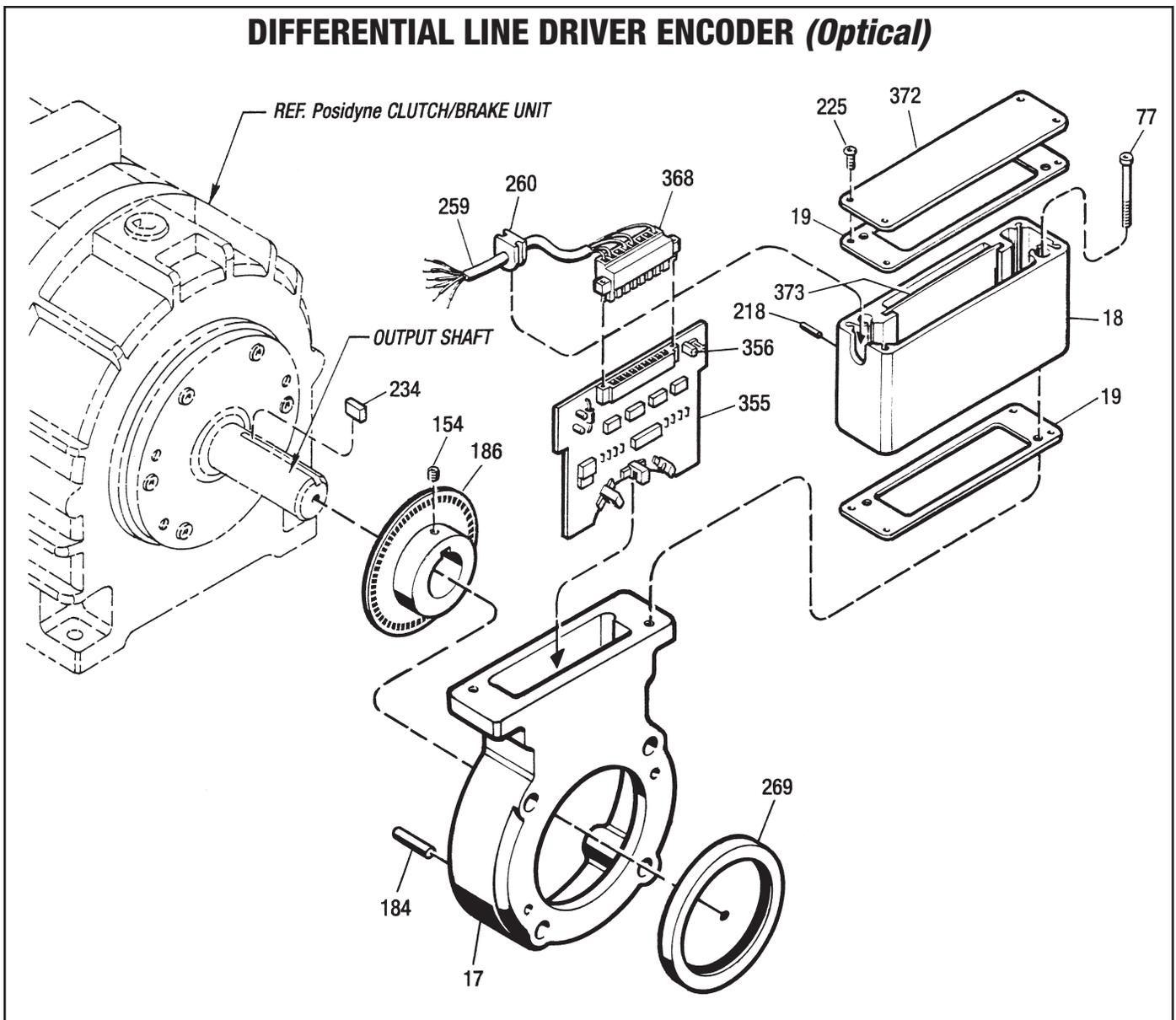
Figure 10.8 - Differential Line Driver Encoder (Optical)
