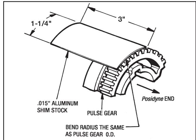
Figure 9.16 - Sensor Gap Shim
