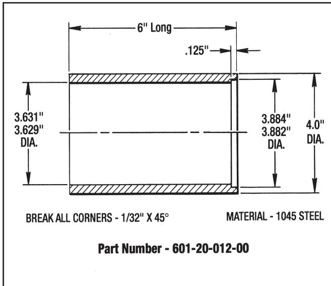
Figure 9.23 - Wear Sleeve (#874) Assembly Tool
