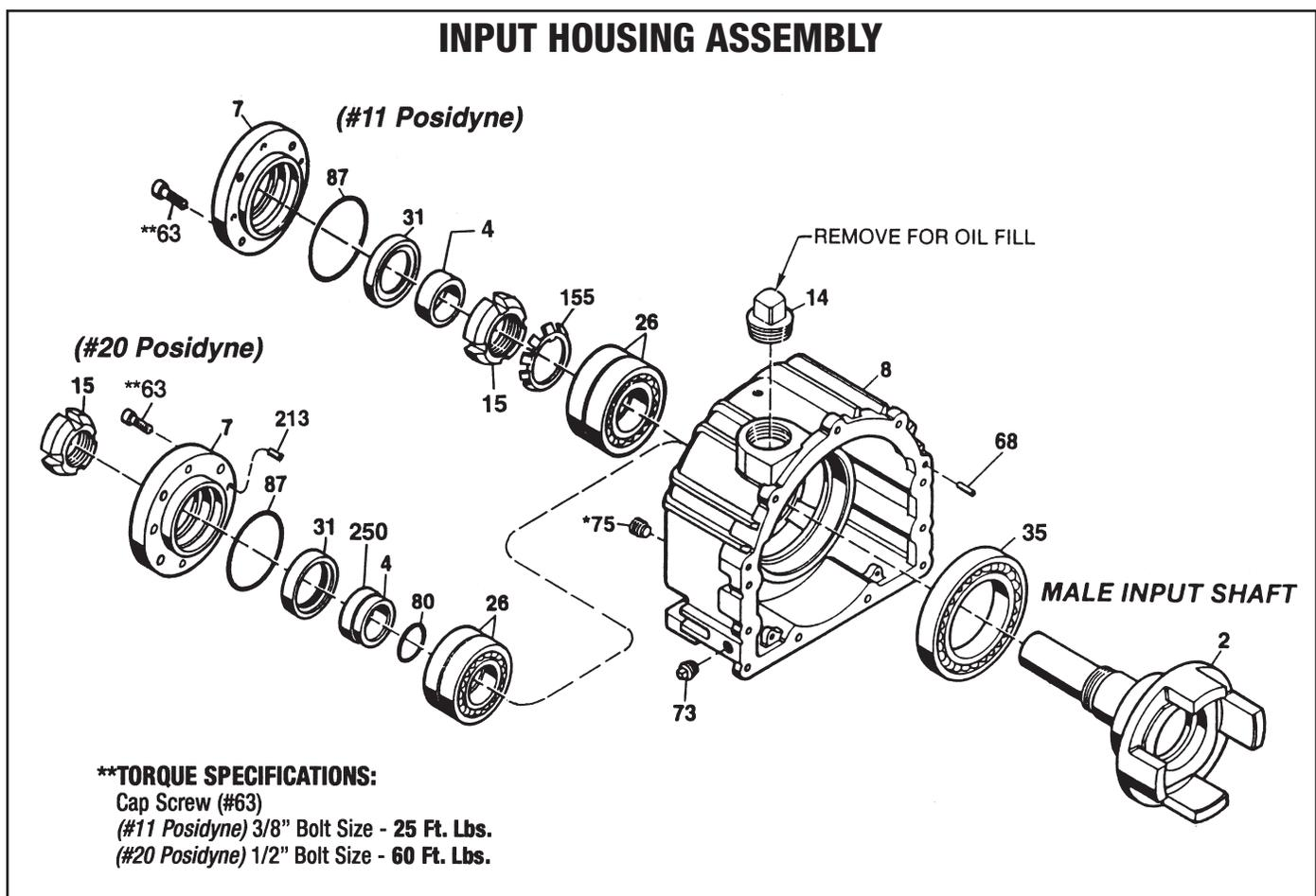
Figure 10.3 - Input Housing Assembly
