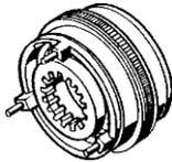
1. Apply (**Loctite #620**) Bearing Retainer Compound to the O.D. of Bearing (#27) and lightly press it into the Piston (#3).
