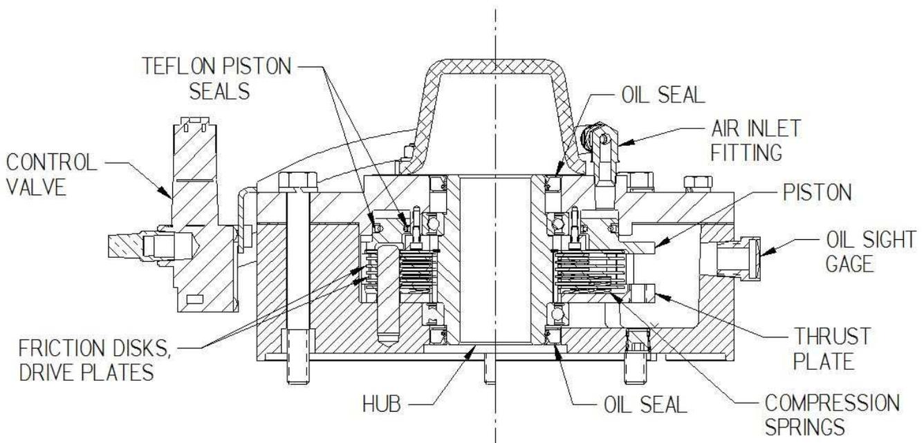
Figure 1.2 - Curing Press Brake Section
