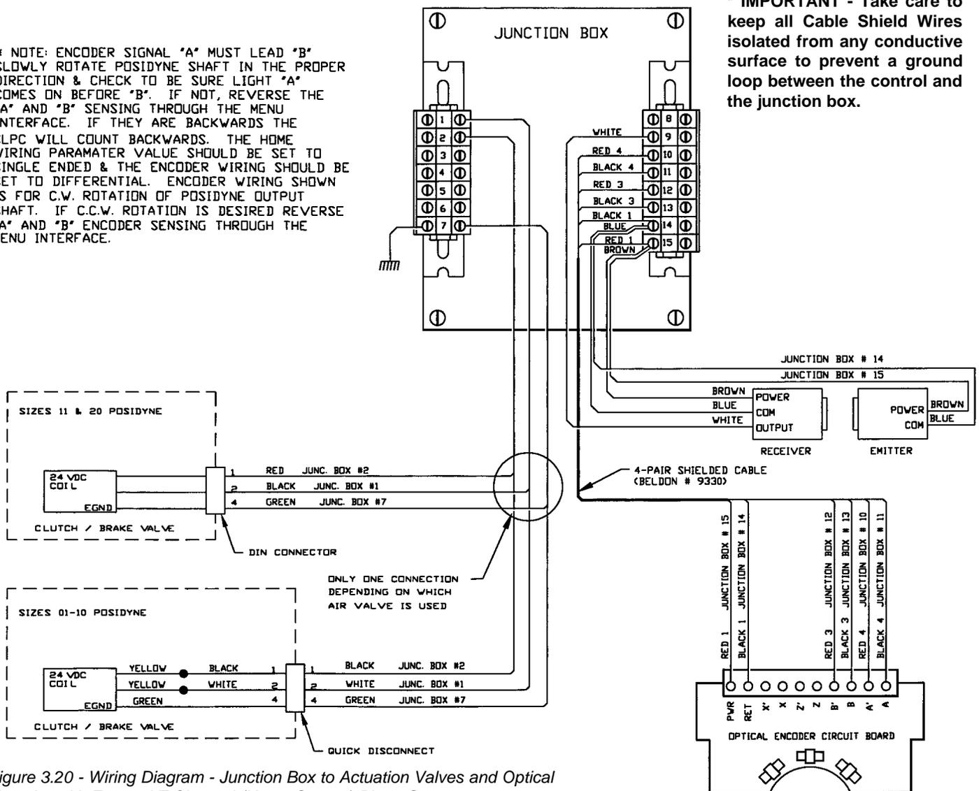
Figure 3.20 - Wiring Diagram - Junction Box to Actuation Valves and Optical Encoder with External Z Channel (Home Sensor) Photo Sensor
