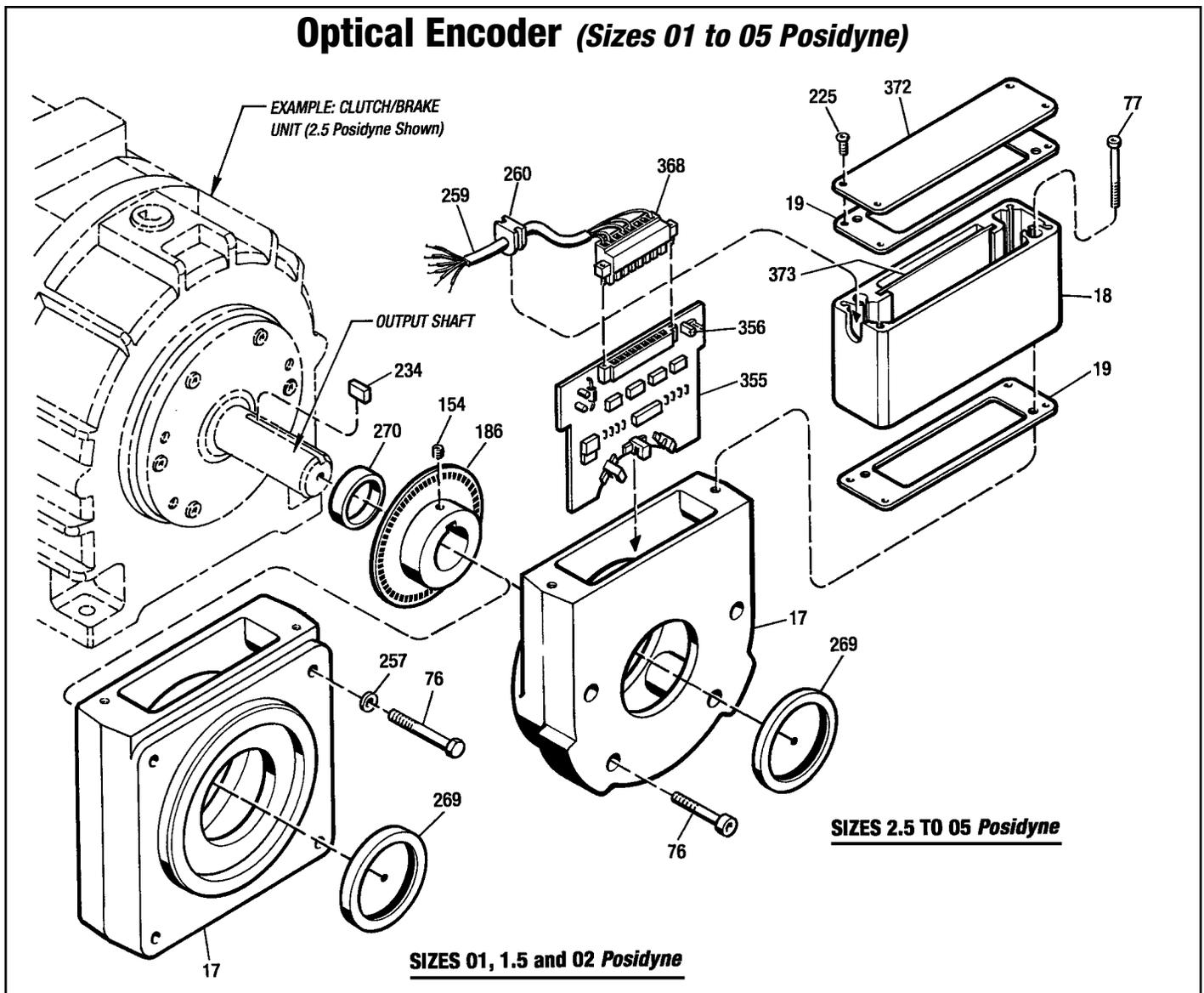
Figure 7.3 - Optical Encoder - (Sizes 01 to 05 Posidyne)
