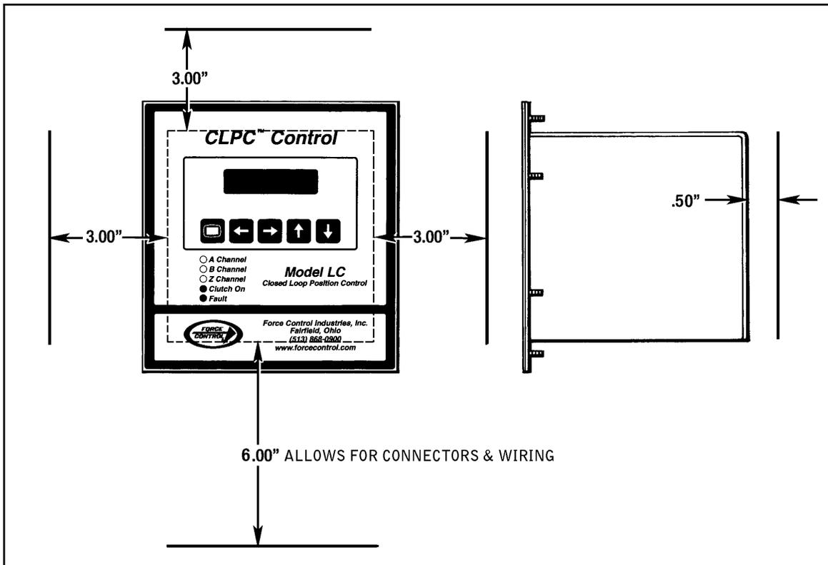
Figure 3.3 - Minimum Mounting Clearances
