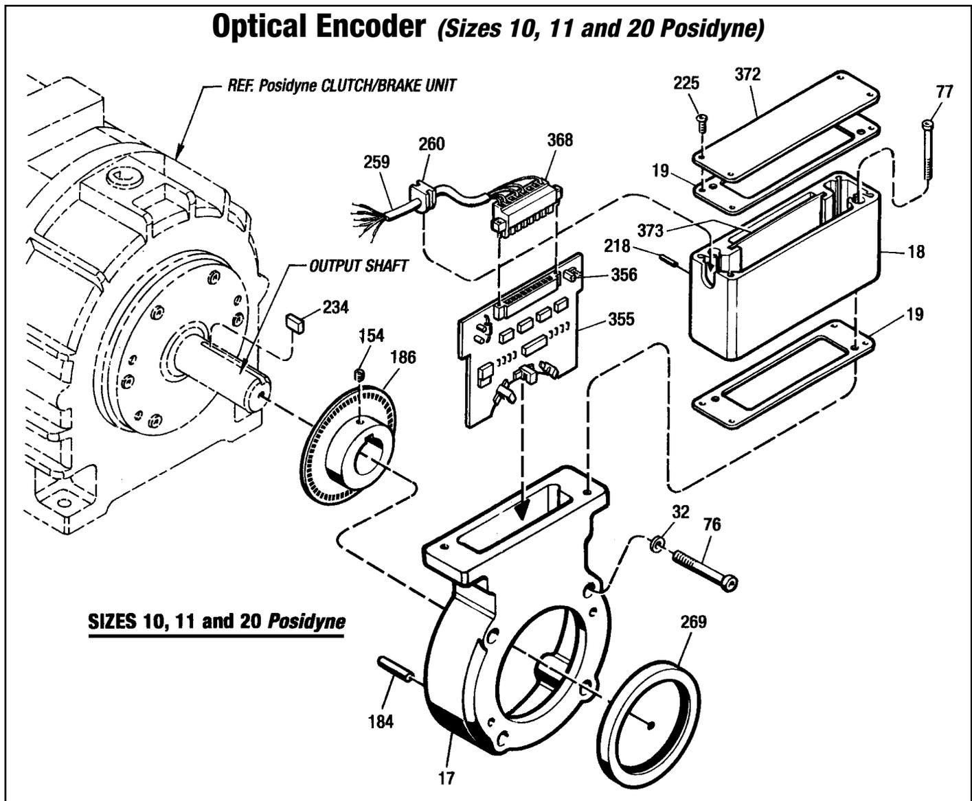
Figure 7.4 - Optical Encoder - Sizes 10, 11 and 20 Posidyne
