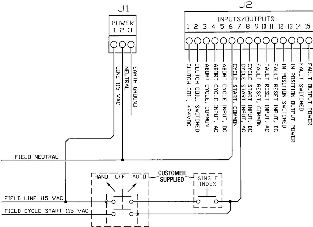
Figure 3.9 - Cycle Start/Hand Off Auto/Single Index (115 VAC)
