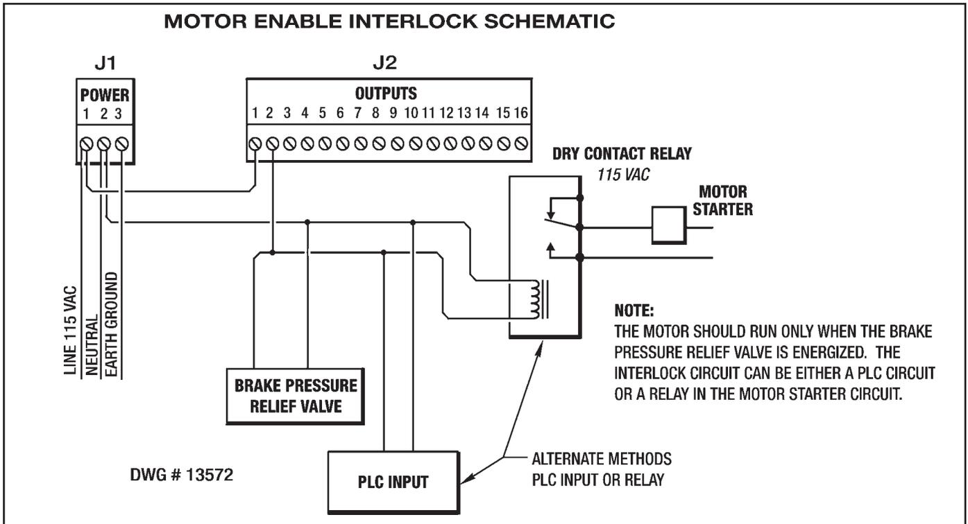
Figure 2.5 - Motor Interlock Schematic
