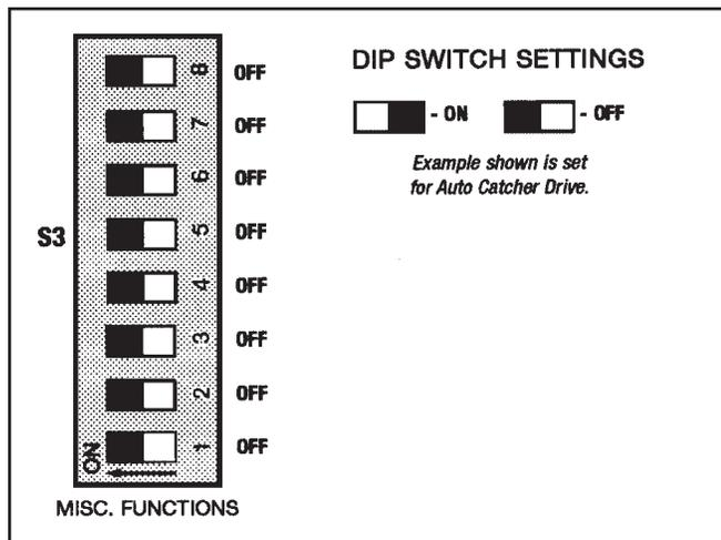
Figure 3.8 - Setting Misc. Functions (Dip Switch #S3)
