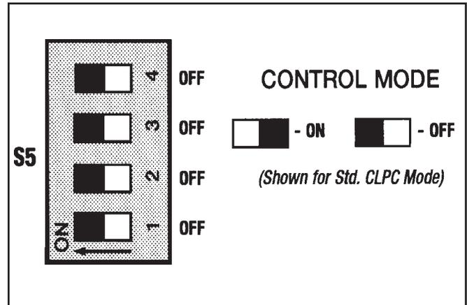
Figure 3.6 - Setting Dip Switch S5 (Control Mode)
