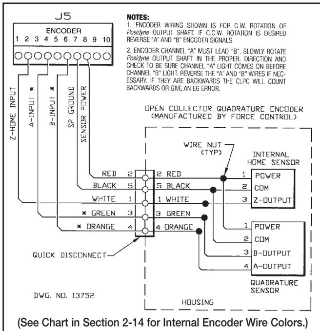
Figure 2.9 - Wiring Diagram - Terminal Block J5 (Open Collector Quadrature Encoder with Internal Home Sensor)
