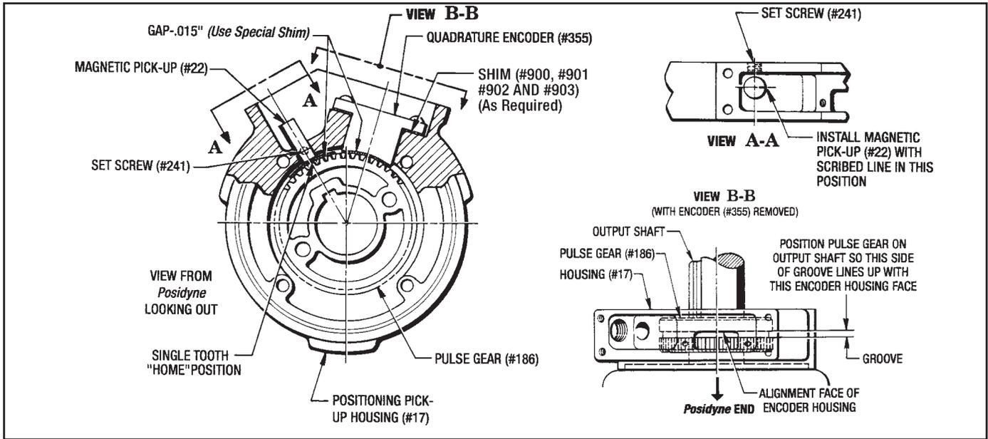
Figure 6.6 - Position Sensors Installation
