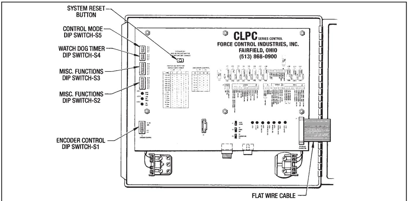
Figure 3.4 - CPU Board Component Location
