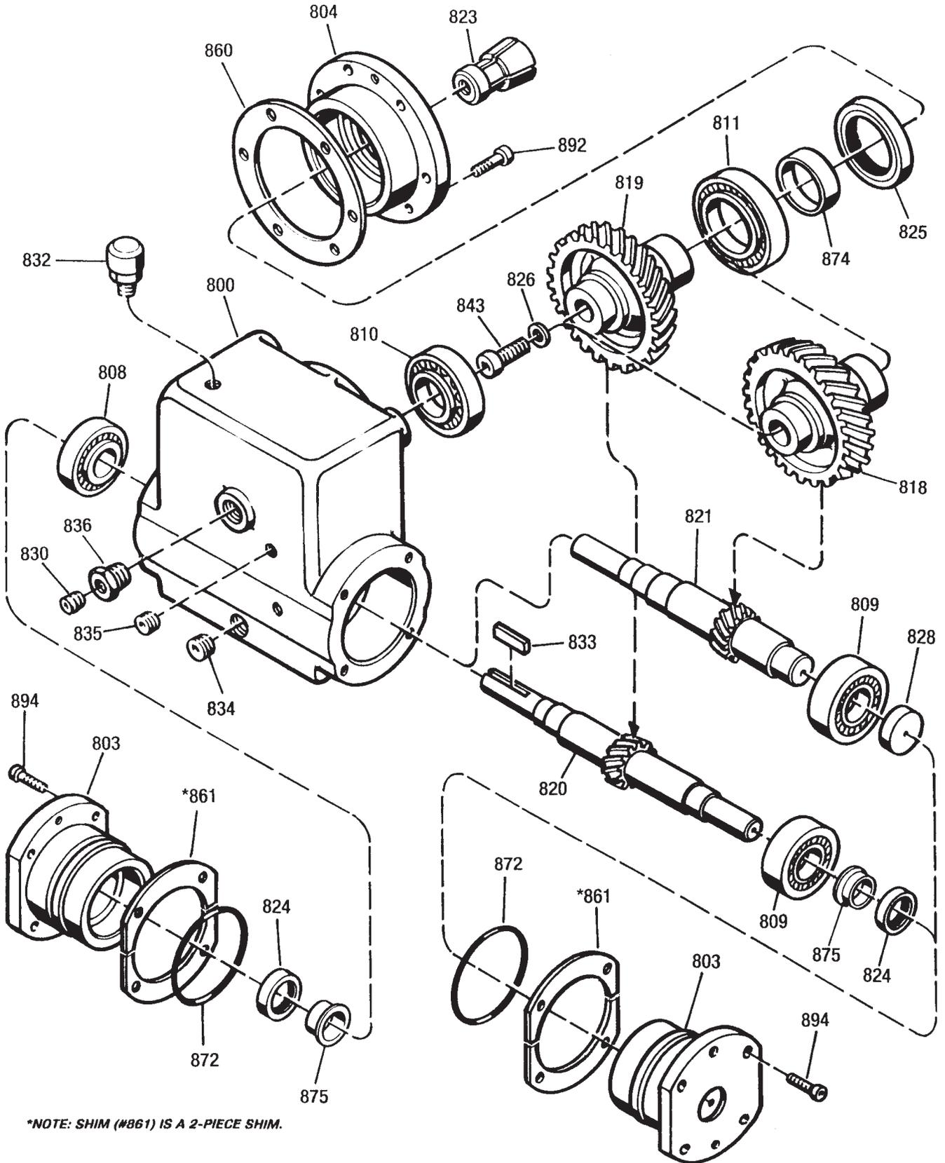
Figure 7.5 - Starwheel Gearbox Assembly
