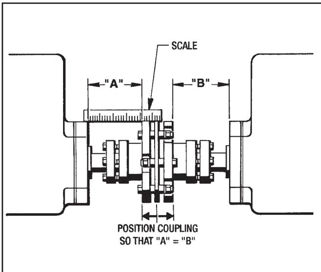
Figure 6.11 - Coupling Alignment
