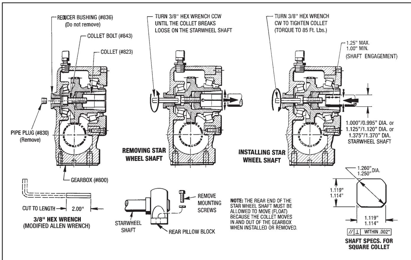
Figure 2.2 - Installing Starwheel into the Gearbox Collet
