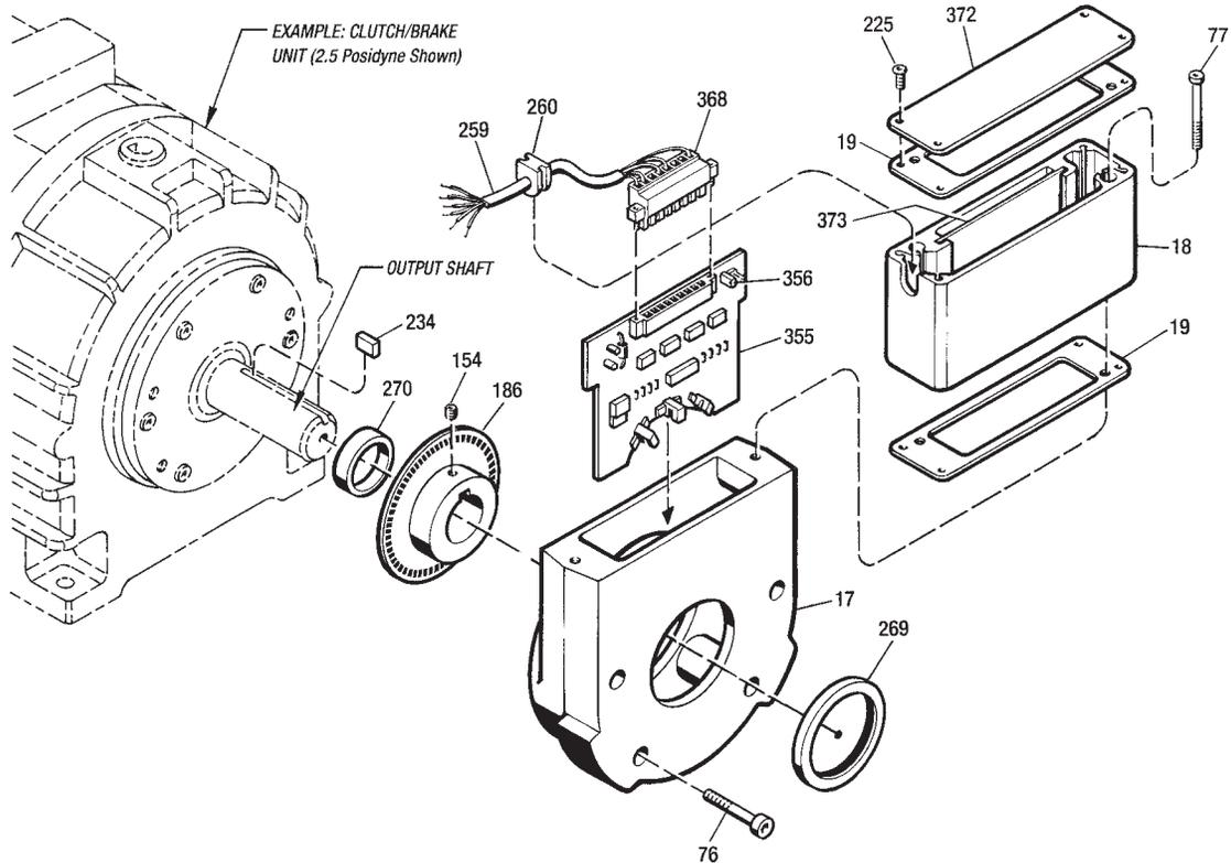
Figure 7.4 - Differential Line Driver (Optical) Encoder
