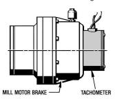
Tachometers or Encoders can be mounted to the end housing of the *Posistop* Brake.
