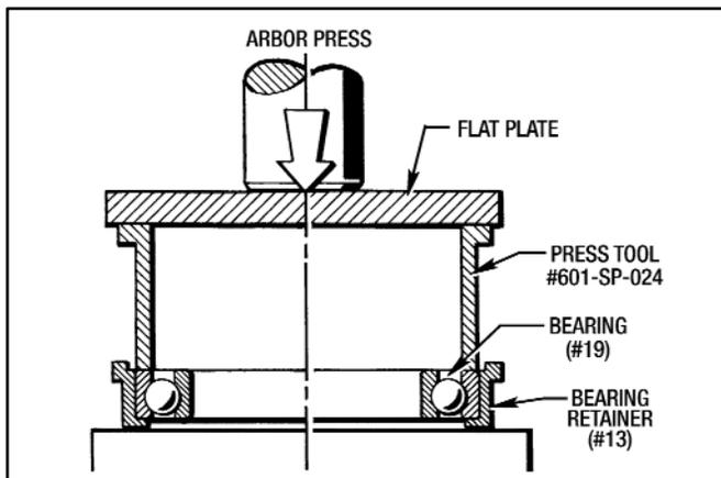
Figure 7.1 - Installing Bearing (#19) into Bearing Retainer (#13)
