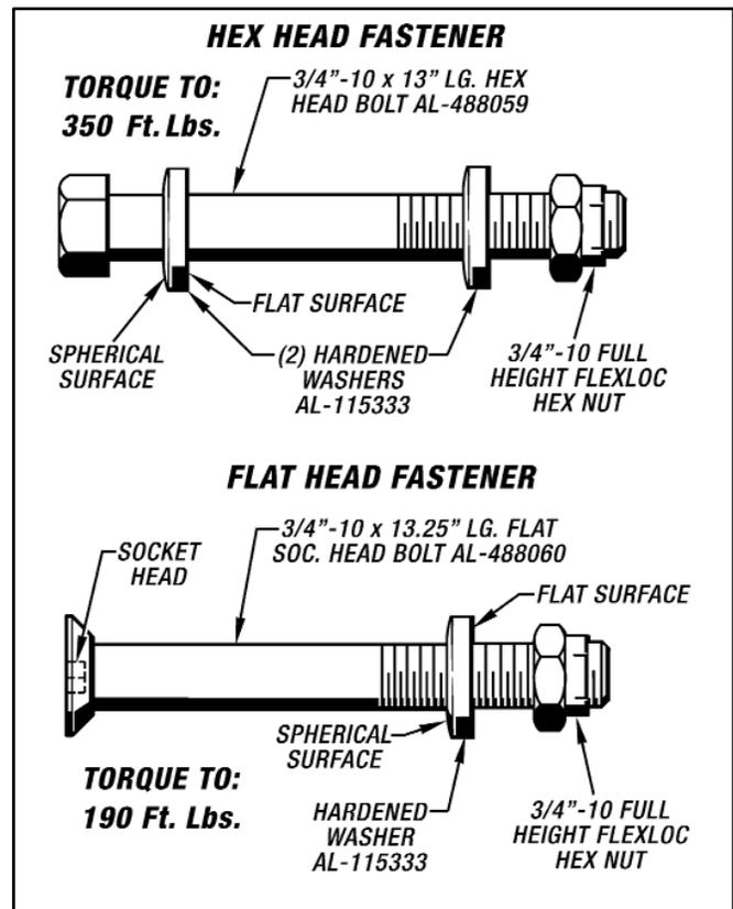
Figure 4.3 - Ultracpac Fastening System
