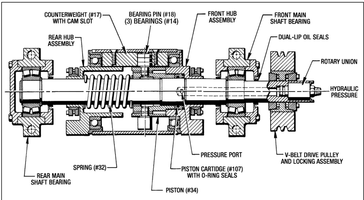
Figure 1.2 - Cross Section thru SmartPac Vibrator Shaft
