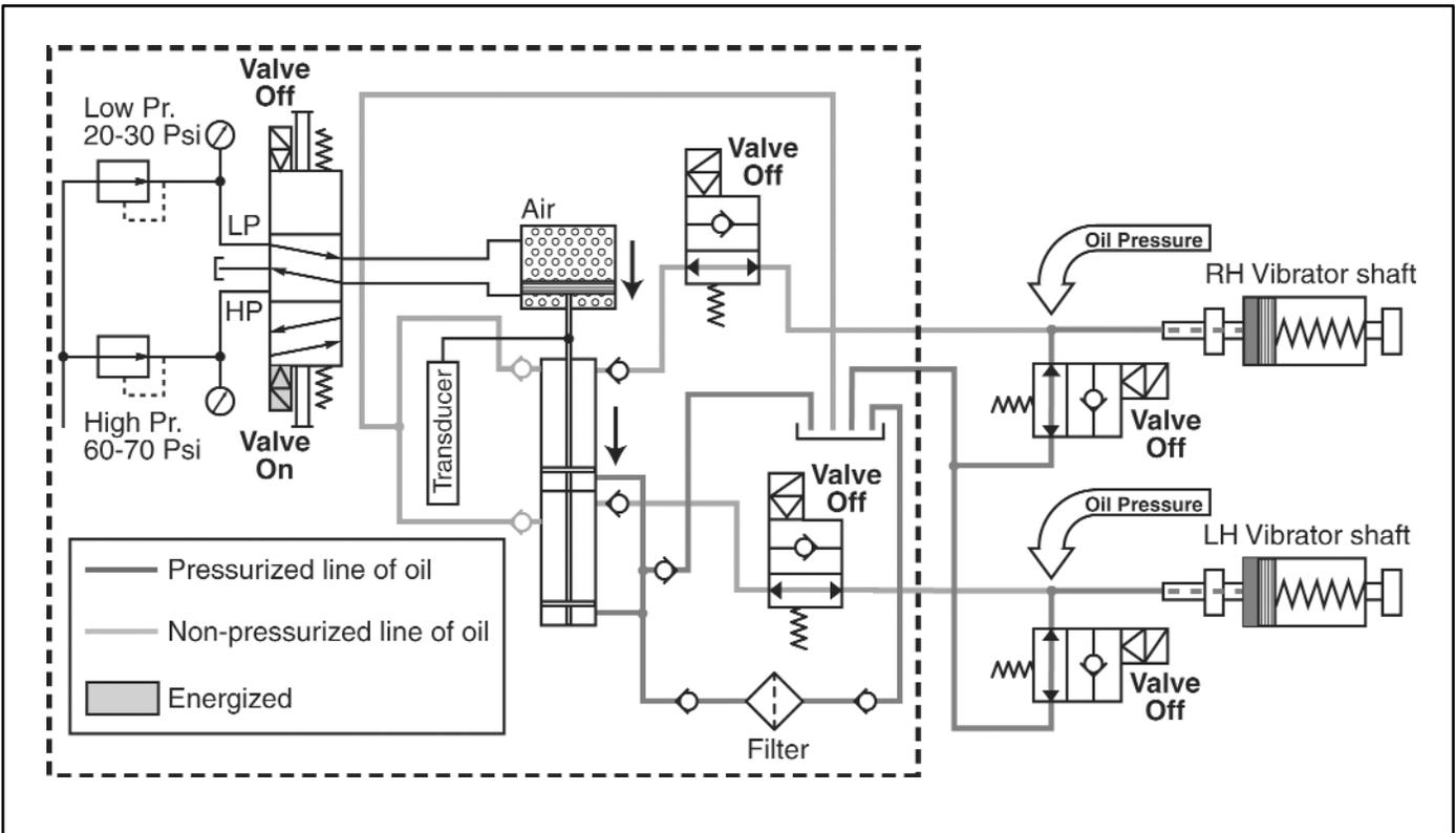
Figure 10.3 - Air-Hydraulic System Diagram - Vibration Off
