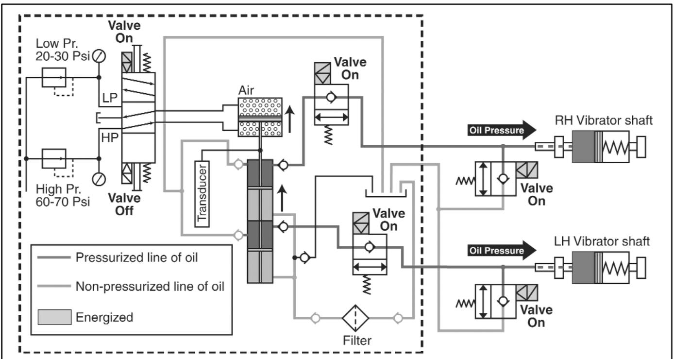
Figure 10.2 - Air-Hydraulic System Diagram - Vibration On/Half Stroke (Amplitude)
