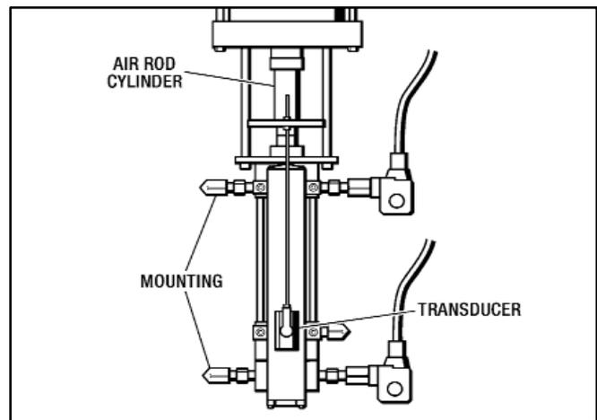
Figure 5.2 - Transducer Adjustment
