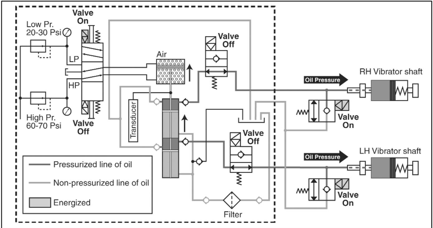
Figure 10.1 - Air-Hydraulic System Diagram - Vibration On/Full Stroke (Amplitude)
