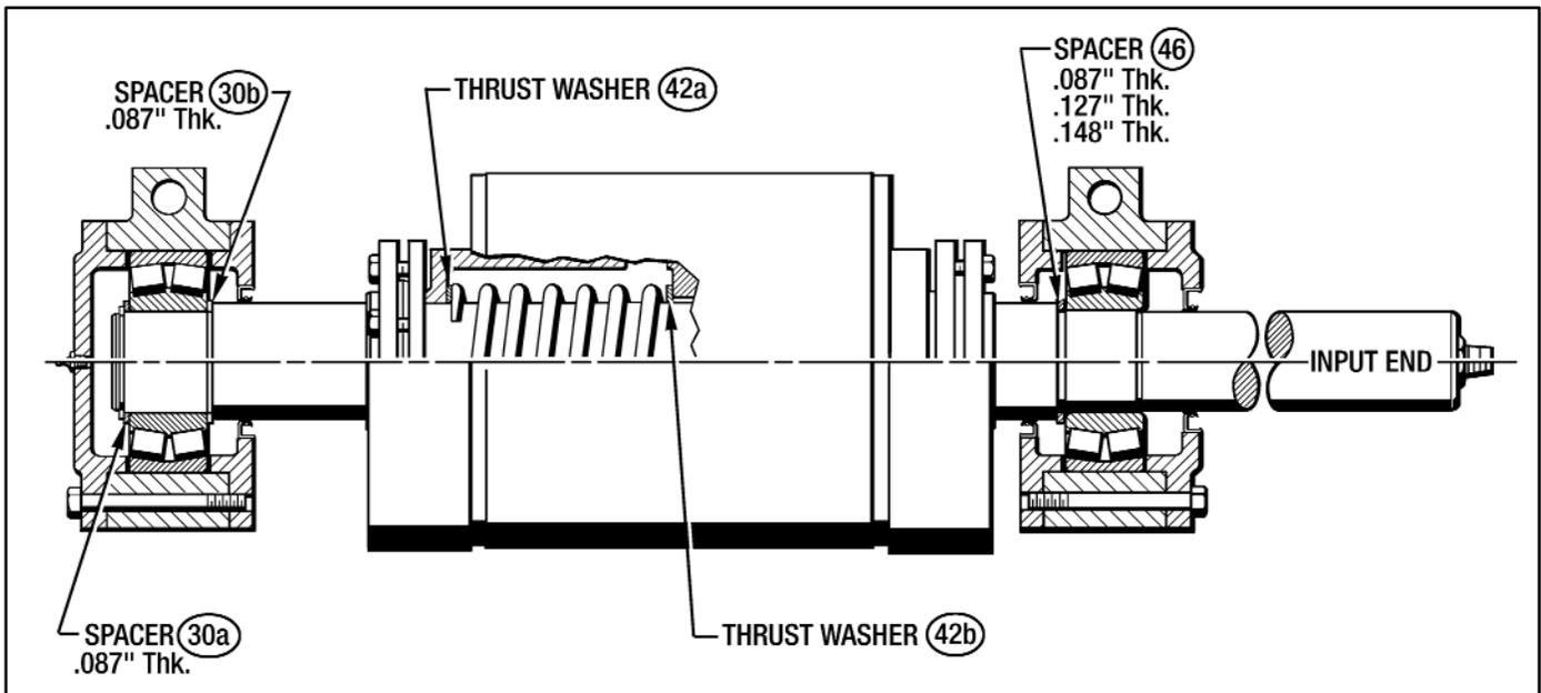
Figure 8.5 - Spacers and Thrust Washer Usage
