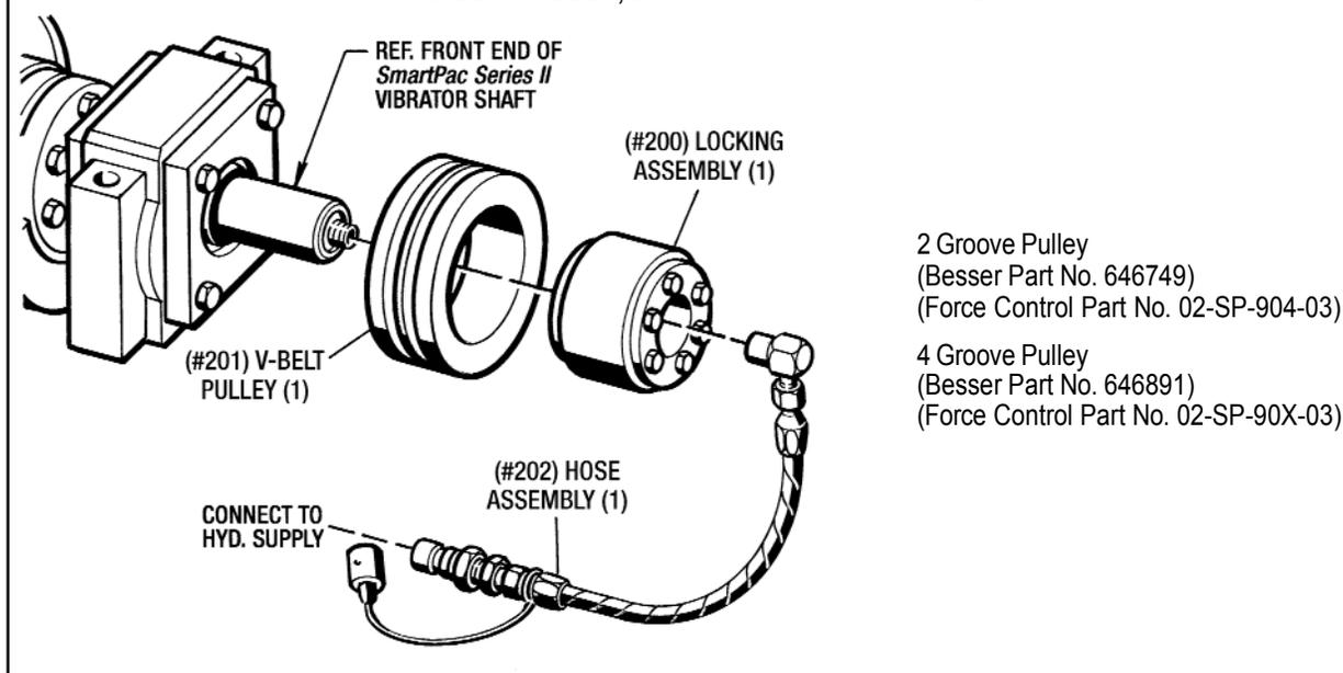
Figure 8.3 - V-Belt Pulley and Hose Assembly Kit
