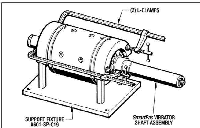
Figure 6.4 - L-Clamps and Support Fixture #601-SP-019
