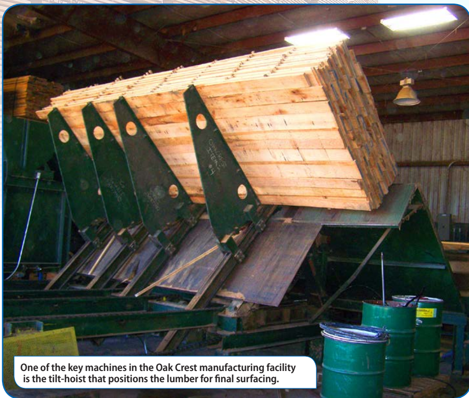
The original drive system of the Oak Crest's tilt-hoist included a dry friction clutch-brake.
