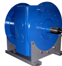
Positorq Drawworks Brake Hydraulically Actuated Brake 150,000 Lb. Ft. Static Torque 70,000 Lb. Ft. Continuous Slip
