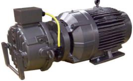
ter hub out through the friction stack both transmits torque without physical wear on the friction discs, and removes the heat of engagement to the housing for dissipation. This nearly eliminates friction disc wear, requires no adjustment, and last with minimal service (check fluid level and change annually) for many years.
