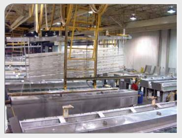
Before employing oil-shear technology, Linetec's service team constantly had to repair the company's anodizing system's brakes from scissor-lifts hoisted 30 feet in the air. The new system has dramatically reduced brake maintenance.
