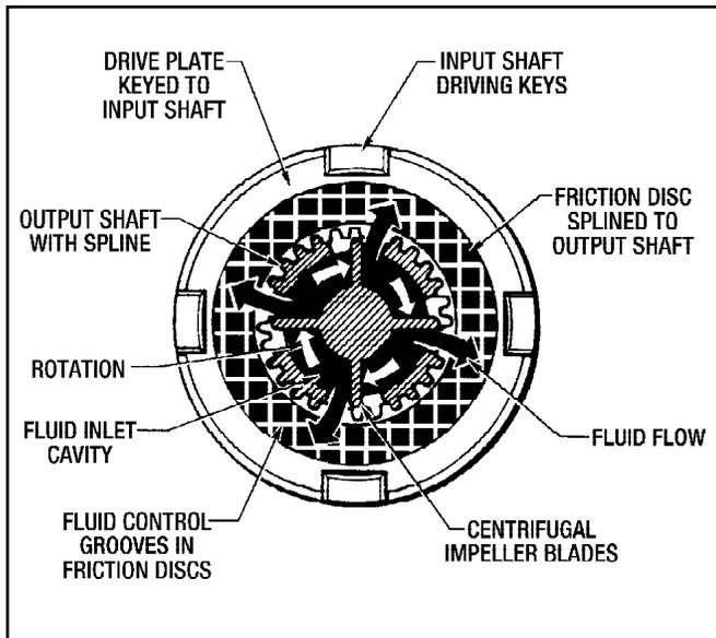
Figure 1.4 - The Oil Shear System
