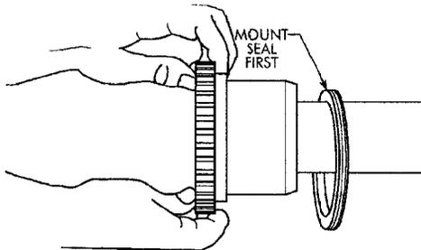
Lock out starting switch of prime mover. Clean all metal parts using a non-flammable solvent. Lightly coat seals with grease and place on shafts BEFORE mounting hubs. Heat interference fit hubs as previously instructed. Seal keyways to prevent leakage. Mount hubs on their respective shafts so the hub face is flush with the end of its shaft unless otherwise indicated. Tighten setscrews when furnished.
