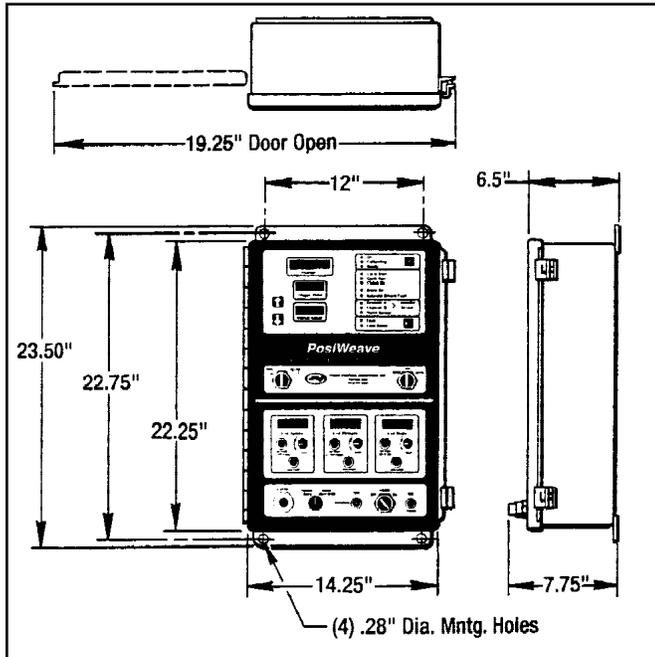
Figure 2.4 - *PosiWeave* Control Box Mounting
