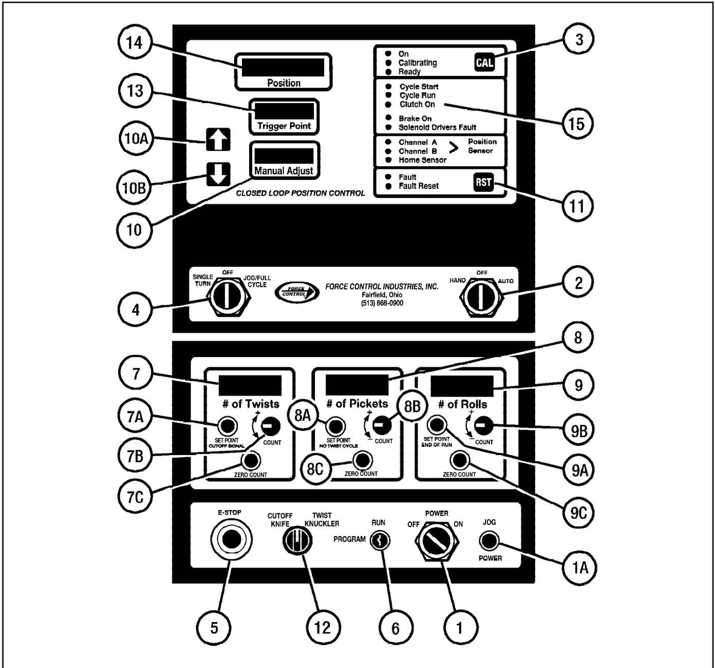
Figure 3.1 - Front PosiWeave Control Panel
