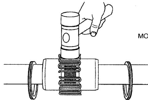
Pack gap and grooves with specified lubricant before inserting grid. When grids are furnished in two or more segments, install them so that all cut ends extend in the same direction (as detailed in the exploded view picture above); this will assure correct grid contact with non-rotating pin in cover halves. Spread the grid slightly to pass over the coupling teeth and seat with a soft mallet.
