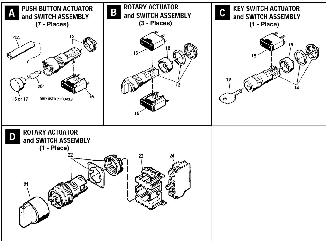
Figure 8.9 - Switch and Actuator Assemblies
