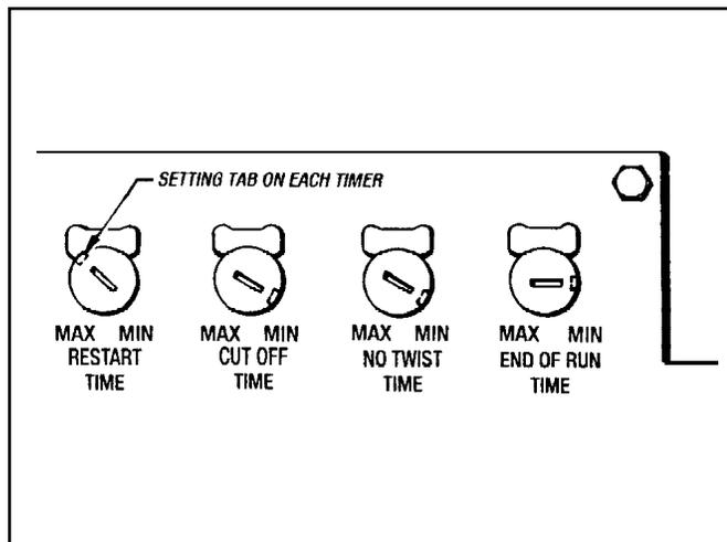
Figure 4.1 Setting Cycle Timers
