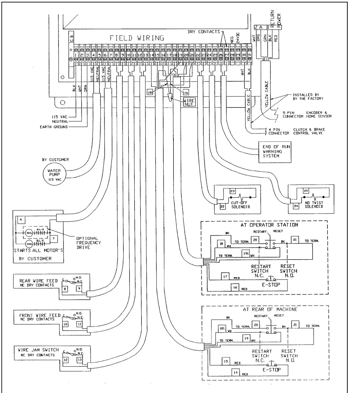
Figure 2.7- Field Wiring Diagram (Pneumatic Actuation with Rear Remote Station)
