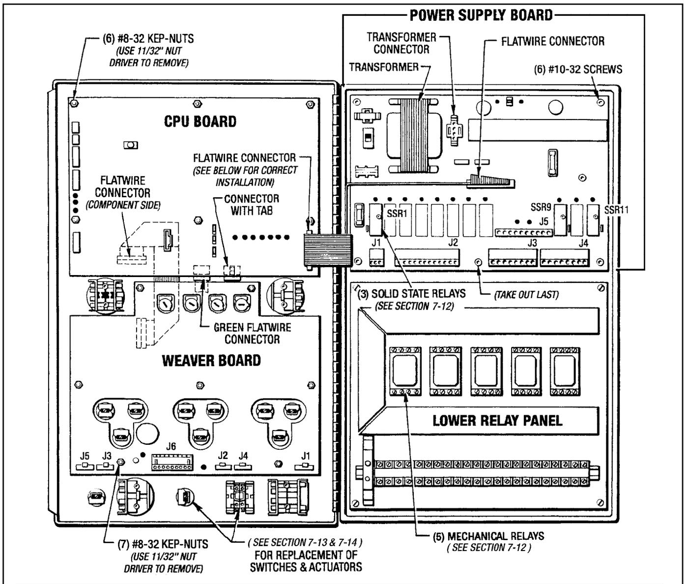
**CORRECT INSTALLATION OF INTER-CONNECTING CABLE**
