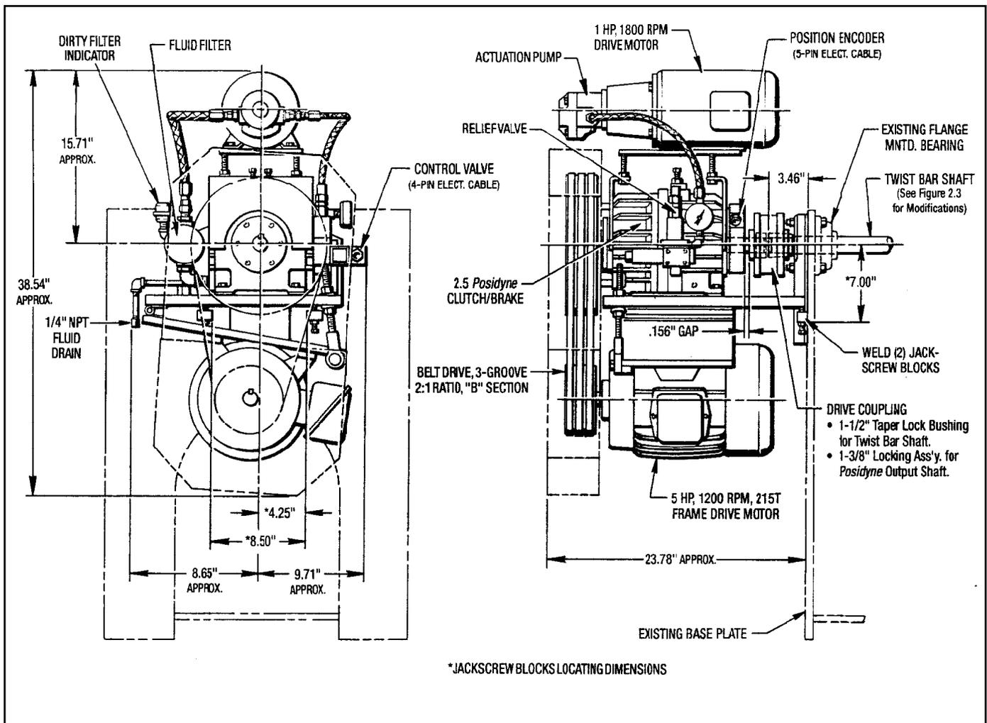
Figure 2.2 - Drive Base Installation (Hydraulic Actuated Drive)
