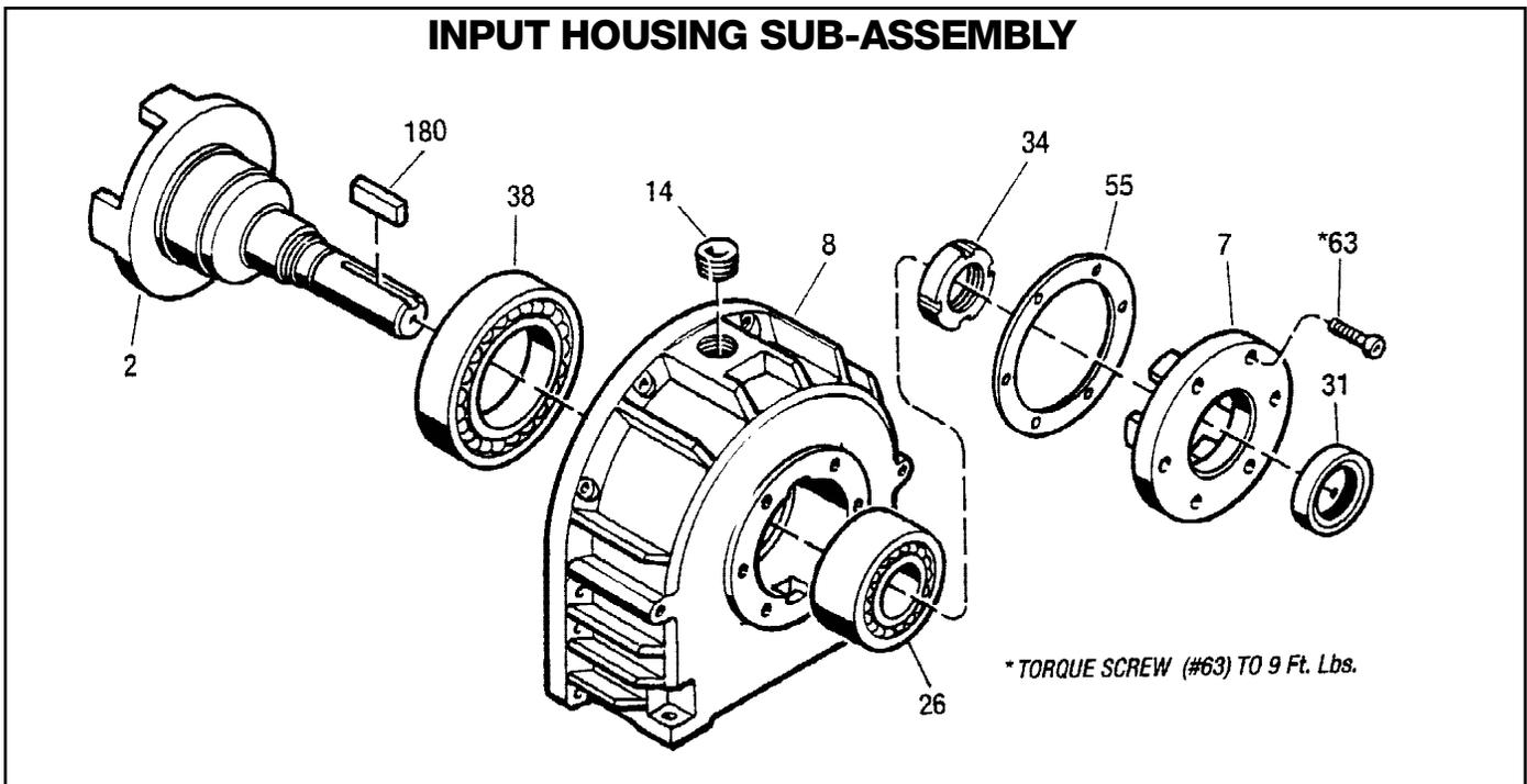
Figure 8.2 - Input Housing Sub-Assembly
