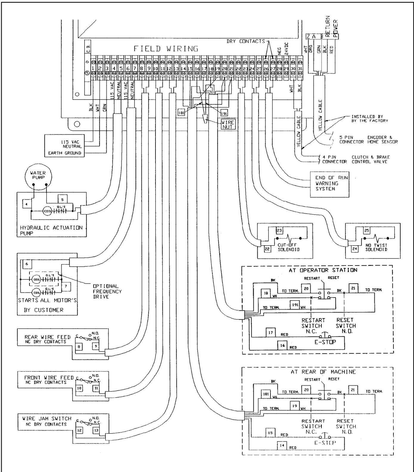
Figure 2.9 - Field Wiring Diagram (Hydraulic Actuation with Rear Remote Station)
