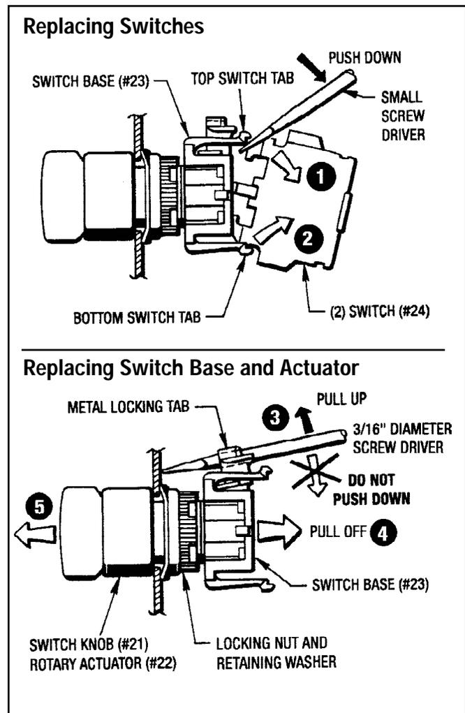
Figure 7.9 - Replacing "Cutoff Knife/Twist Knuckler" Switch
