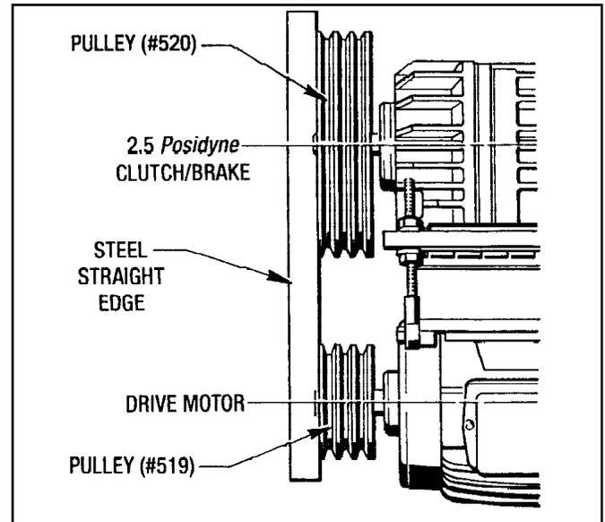
Figure 7.5 - Pulley Alignment
