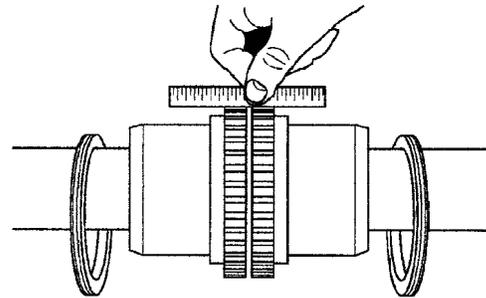
Align so that a straight edge rests squarely (or within the limits specified in Table 2) on both hubs as shown above and also at 90° intervals. Check with feelers. The clearance must not exceed the PARALLEL OFFSET installation limits specified in Table 2. Tighten all foundation bolts and repeat Steps 2 and 3. Realign coupling if necessary.
