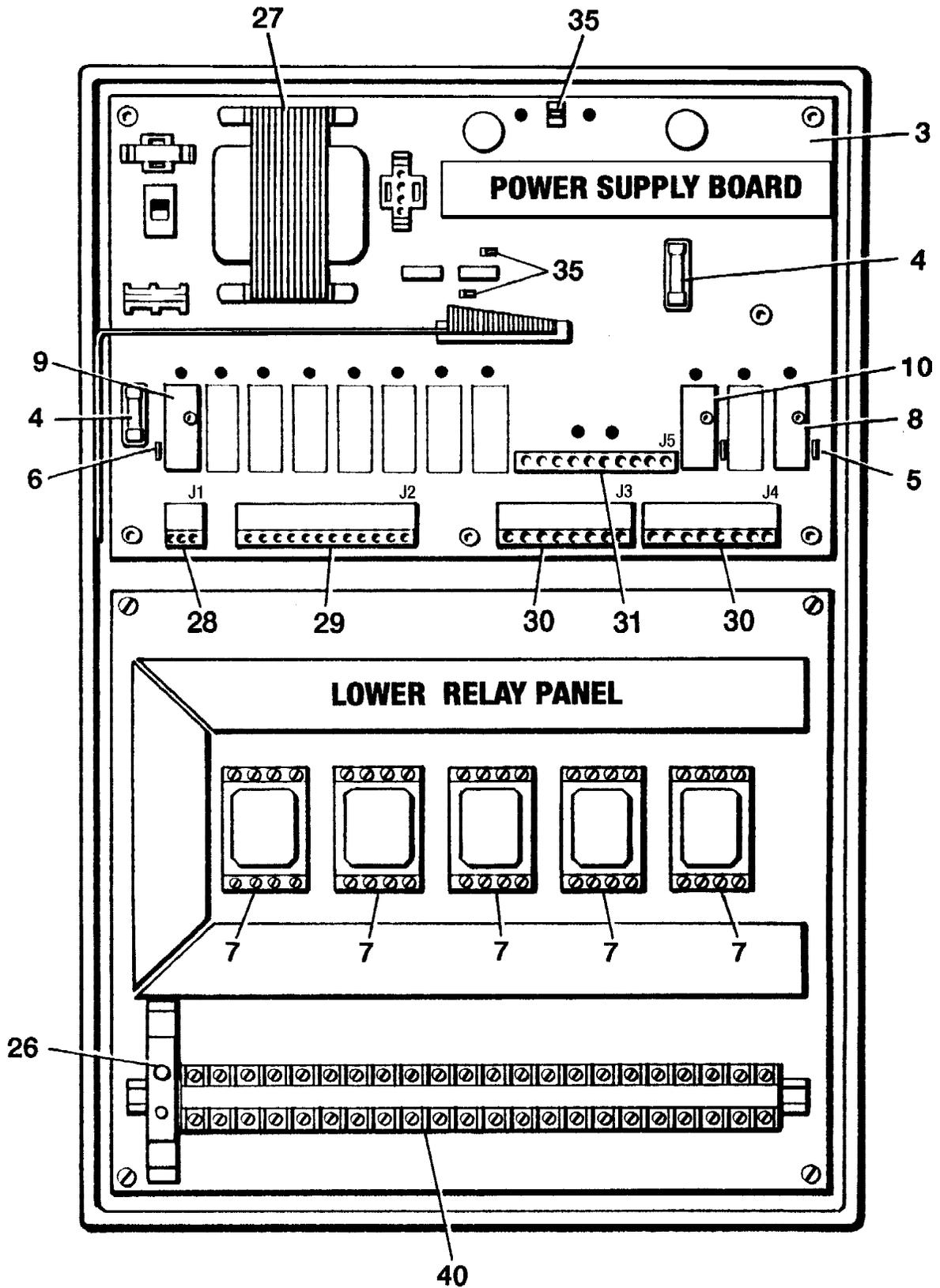
Figure 8.11- Power Supply Board and Lower Relay Panel
