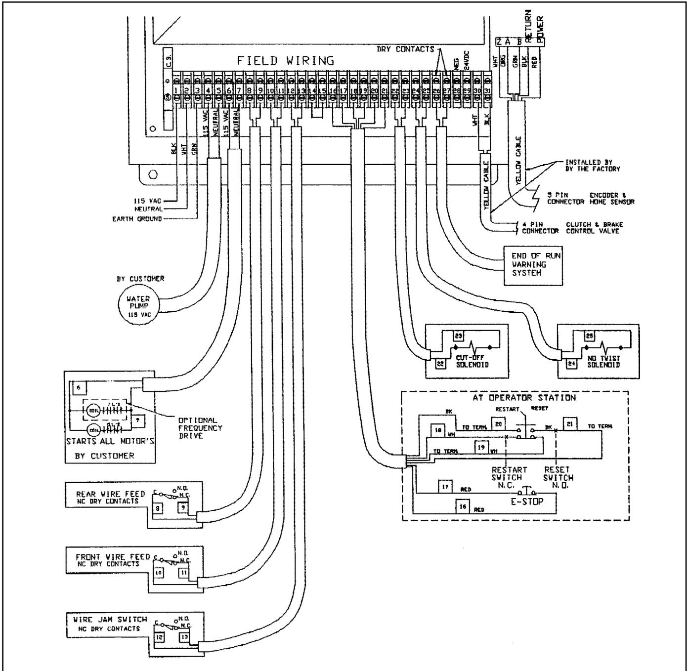
Figure 2.6 - Field Wiring Diagram (Pneumatic Actuation without Rear Remote Station)
