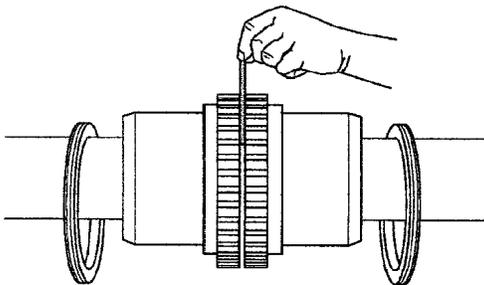
Use a spacer bar equal in thickness to the gap specified in Table 2, Page 5. Insert bar as shown below left, to same depth at 90° intervals and measure clearance between bar and hub face with feelers. The difference in minimum and maximum measurements must not exceed the ANGULAR installation limits specified in Table 2.
