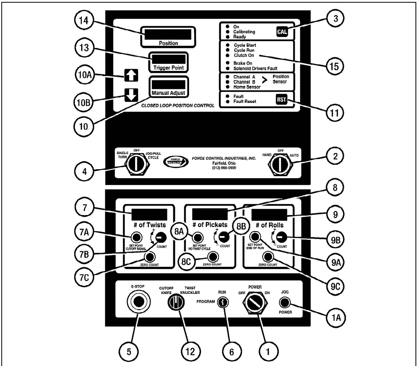
Figure 4.3 - PosiWeave Front Control Panel
