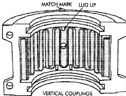
UP or on the high side. Push gaskets in until they stop against the seals and secure cover halves with fasteners, tighten to torque specified in Table 2. Make sure gaskets stay in position during tightening of fasteners. **CAUTION:** Make certain lube plugs are installed before operating.
