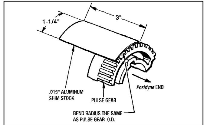
Figure 7.2 - Sensor Gap Shim
