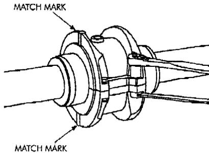
Pack the spaces between and around the grid with as much lubricant as possible and wipe off excess flush with top of grid. Position seals on hubs to line up with grooves in cover. Position gaskets on flange of lower cover half and assemble covers so that the match marks are on the same side (see above). If shafts are not level (horizontal) or coupling is to be used vertically, assemble cover halves with the lug and match mark
