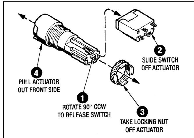
Figure 7.8 - Replacing Actuators and Switches
