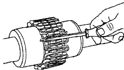
Whenever it is necessary to disconnect the coupling, remove the cover halves and grid. A round rod or screwdriver that will conveniently fit into the open loop ends of the grid is required. Begin at the open end of the grid section and insert the rod or screwdriver into the loop ends. Use the teeth adjacent to each loop as a fulcrum and pry the grid out radially in even, gradual stages, proceeding alternately from side to side.
