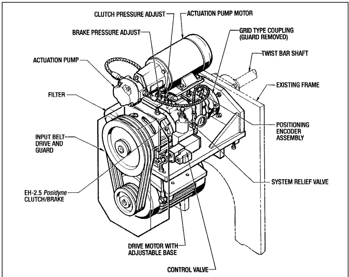
Figure 1.3 - Hydraulically Actuated Drive Package
