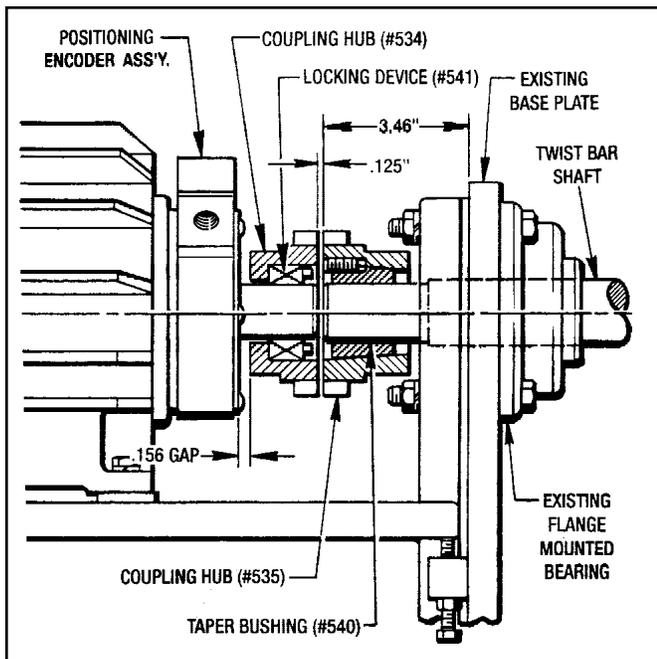
Figure 7.4 - Coupling Installation
