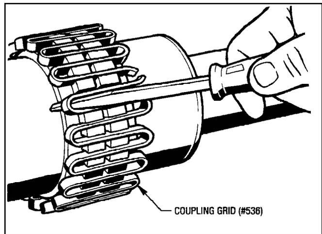
Figure 7.1 - Removing Coupling Grid
