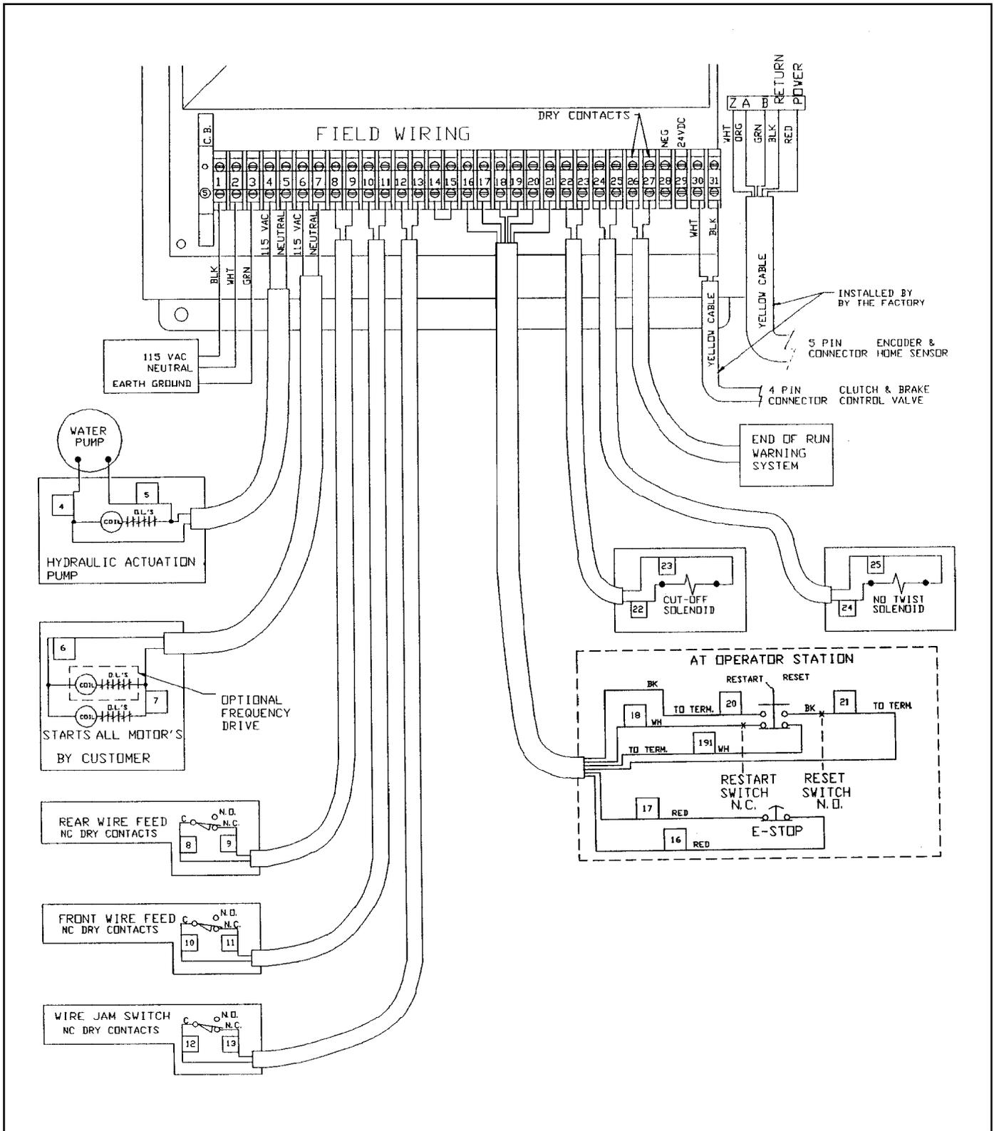
Figure 2.8 - Field Wiring Diagram (Hydraulic Actuation Without Rear Remote Station)
