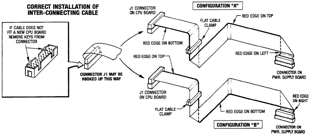
Figure 7.7 - Replacing Circuit Boards
