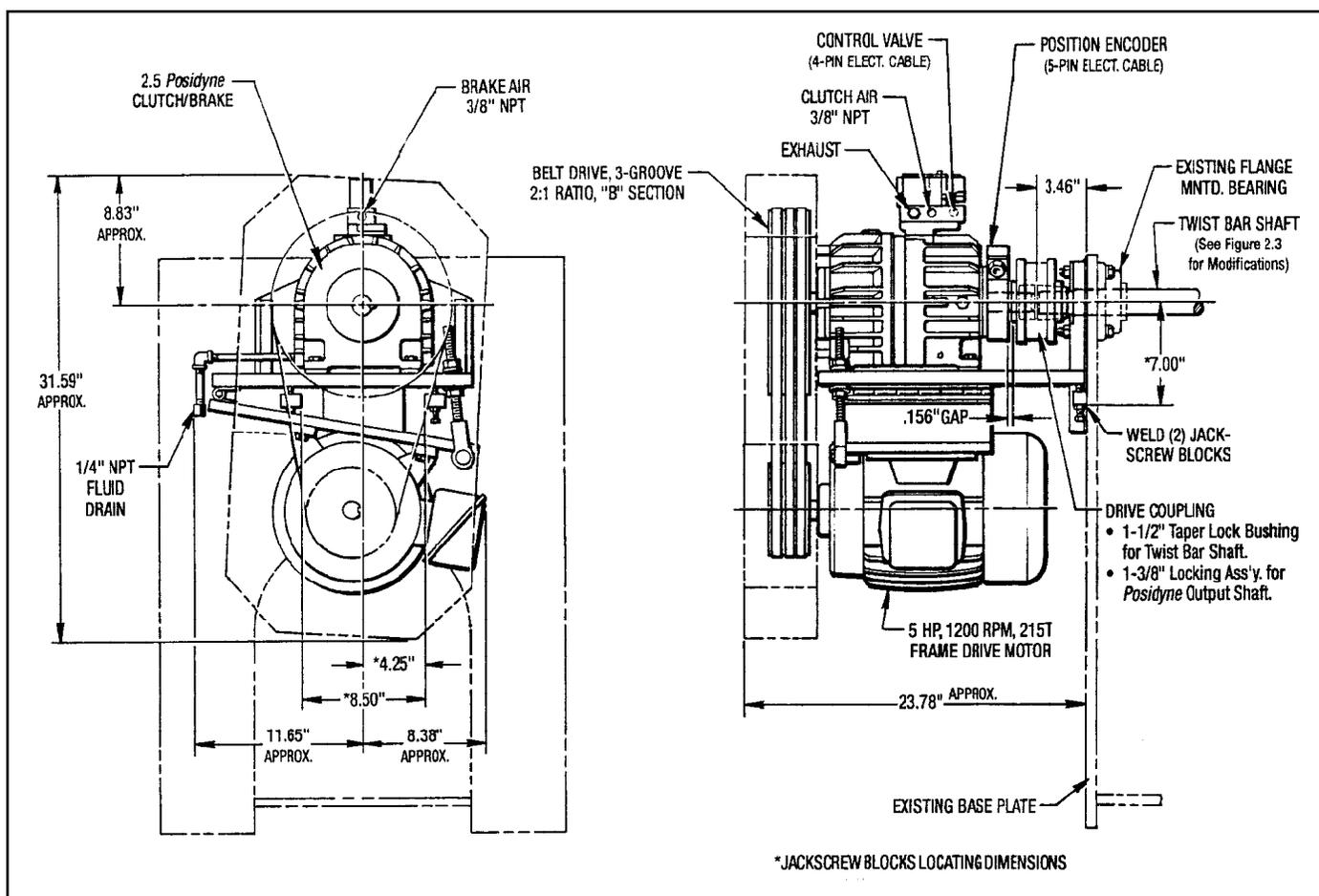
Figure 2.1 - Drive Base Installation (Air Actuated)
