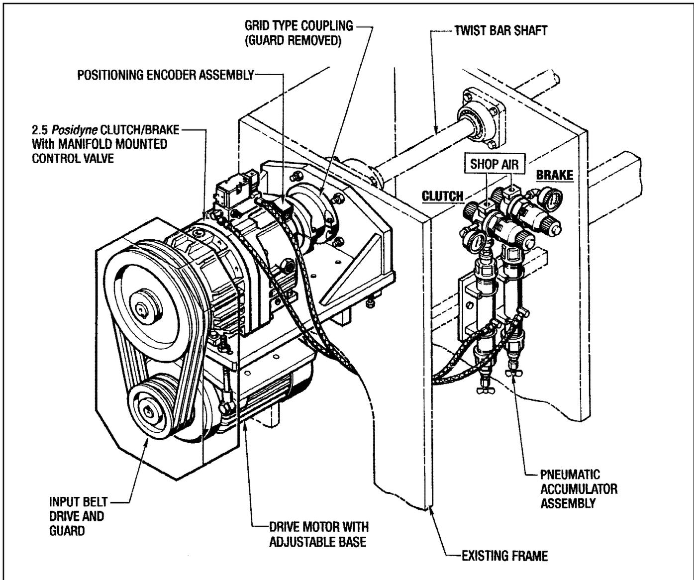
Figure 1.2 - Air Actuated *PosiWeave* Drive Package
