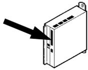
This interface is used to operate the **PosiDrive Series RS** as a slave, mastered by an encoder with 24V-signal level (master-slave operation). The digital inputs DIGITAL-IN 1 and 2 at connector X3 must be used.
