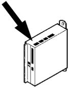
The interface for connecting to the CAN bus (default 500 kBaud). The integrated profile is based on the communication profile CANopen DS301 and the drive profile DSP402. The following functions are available in connection with the integrated position controller: Jogging with variable speed, reference traverse (zeroing), start motion task, start direct task, digital setpoint provision, data transmission functions and many others.
