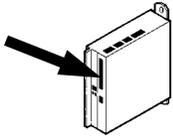
The servo amplifier is equipped with two differential inputs for analog setpoints that are **freely programmable** (with the aid of the macro-language, consult our applications department). Analog Ground (X3/1) must always be joined to the CNC-GND of the controls as a ground reference.
