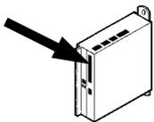
This interface is used to connect the servo amplifier to a stepper-motor controller with 24V-signal level. The digital inputs DIGITAL-IN 1 and 2 at connector X3 must be used.
