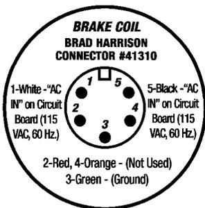
Figure 3.4 - Electrical Connector
