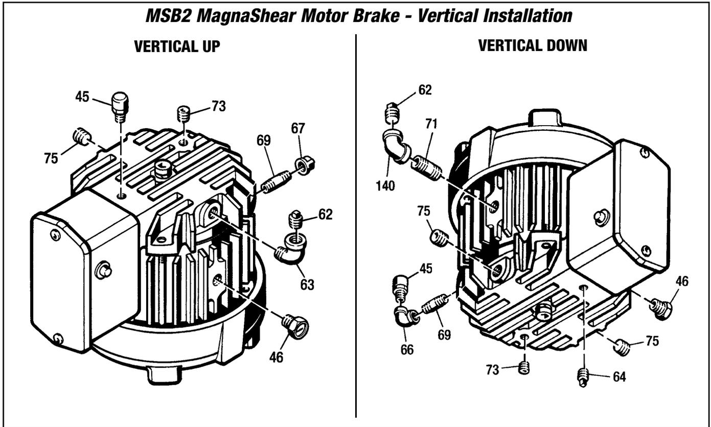
Figure 8.4 - MSB2 MagnaShear Motor Brake - Vertical Installation
