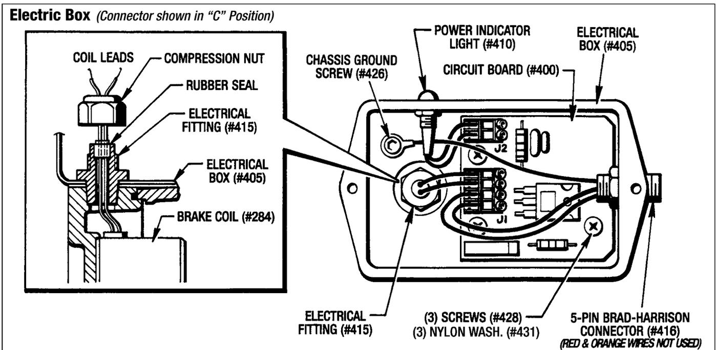
Figure 7.3 - Electric Box with Cover Removed
