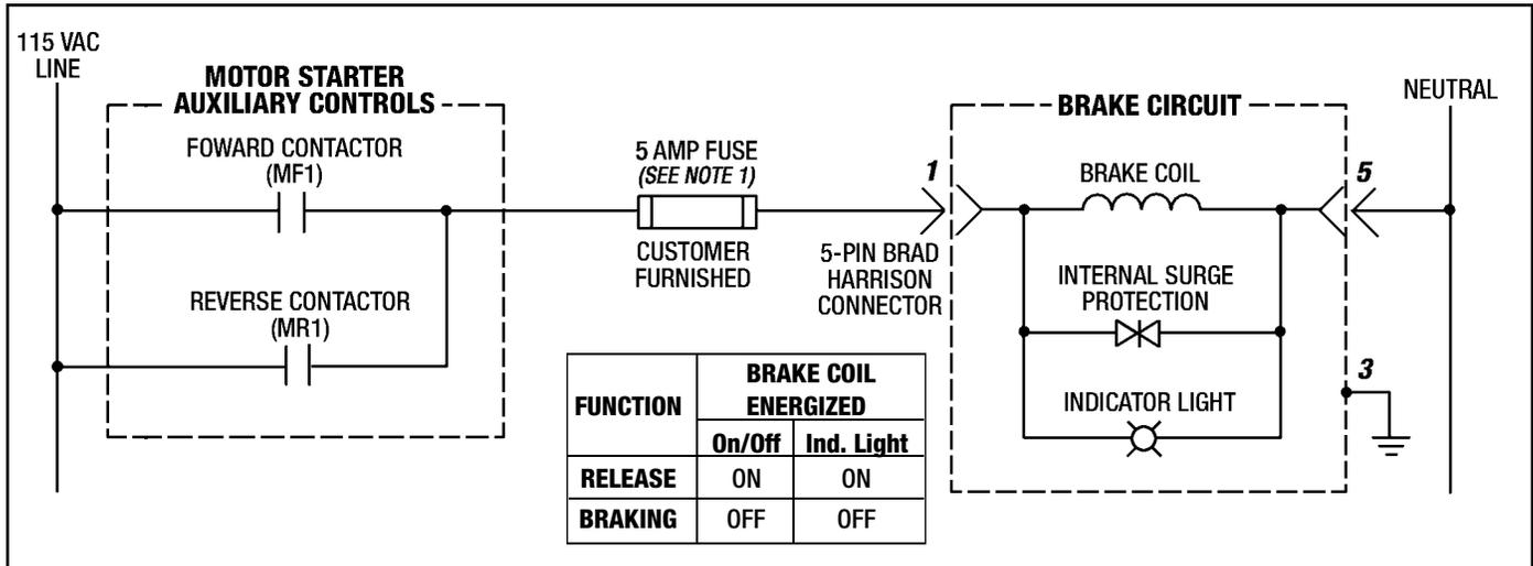
Figure 3.3 - Electrical Schematic
