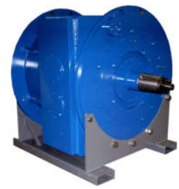
Positorq Large Mooring Winch Brake Hydraulically Actuated Brake 150,000 Lb. Ft. Static Torque 70,000 Lb. Ft. Continuous Slip
