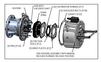
Figure 7.3 - Removing MSB12 Brake Stack
