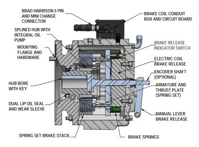
Figure 1 - Unit Description and Operation
