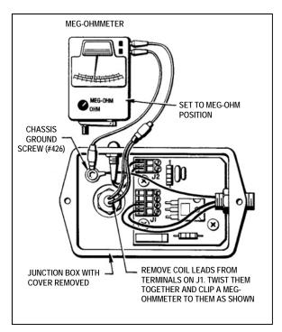
Figure 6.2 - Coil Current Leakage Testing
