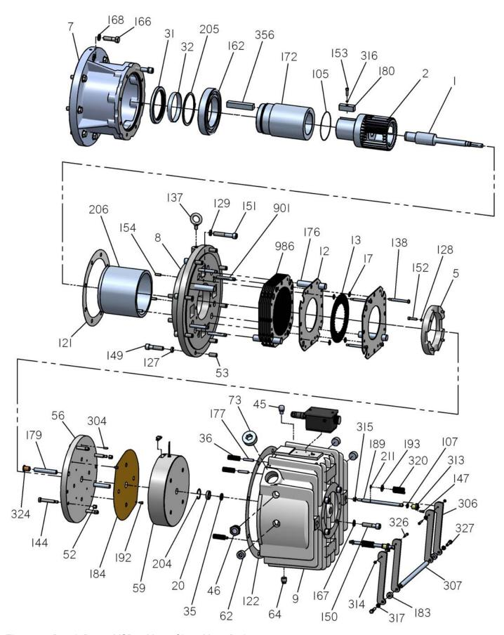
Figure 8.2 Repair Parts - MSB12 MagnaShear Motor Brake
