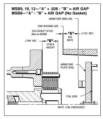
Figure 7.4 - Checking Air Gap for MSB12
