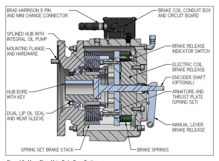
Figure 1.2 - MagnaShear Motor Brake Cross Section
