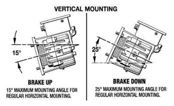
Figure 2 - Vertical Mounting Angles
