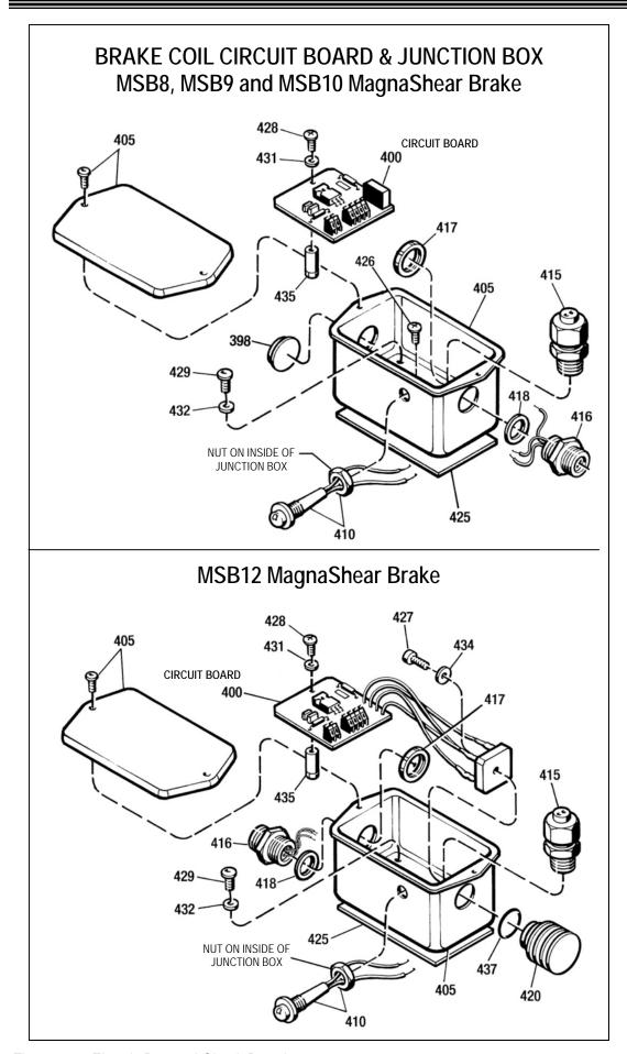
Figure 8.3 - Electric Box and Circuit Board
