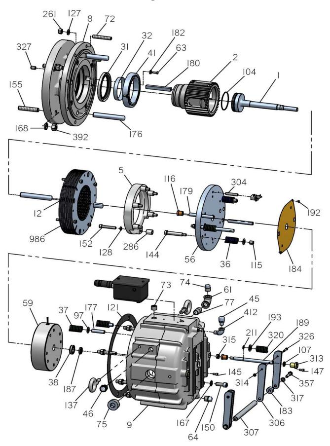
Figure 8.1 - Repair Parts - MSB9 and MSB10 MagnaShear Motor Brake
