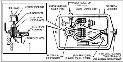
Figure 7.5 - Conduit Box with Cover Removed for Sizes MSB8, MSB9 and MSB10
