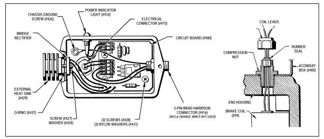
Figure 7.6 - Conduit Box with Cover Removed for Size MSB12 Motor Brake
