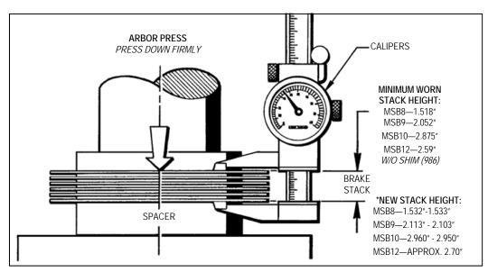
Figure 7.1 - Measuring Stack Height
