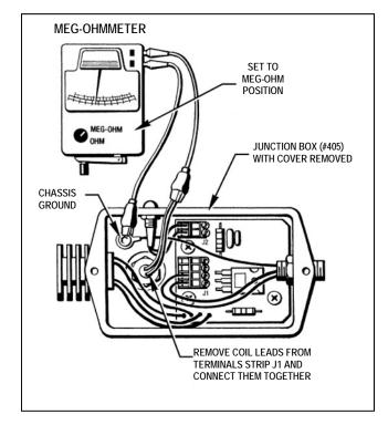
Figure 6.4 - Coil Current Leakage Testing
