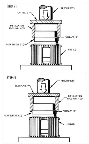
Figure 7.12 - Installing Wear Sleeve (#32) on Sizes MSB9 and MSB10
