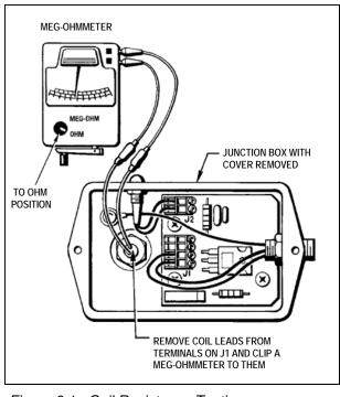
Figure 6.1 - Coil Resistance Testing
