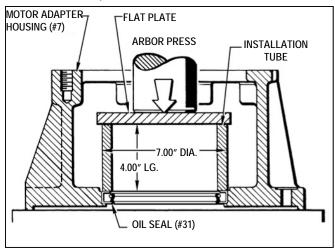
Figure 7.15 - Installing Oil Seal for MSB12
