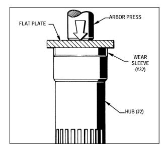
Figure 7.13 - Installing Wear Sleeve (#32) on MSB12
