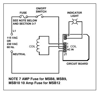
Figure 5.1 - Test Set-Up Electrical Schematic
