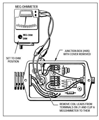
Figure 6.3 - Coil Resistance Testing
