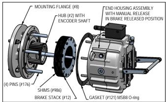
Figure 7.2 - Replacing the Brake Stack (MSB8, MSB9 & MSB10)
