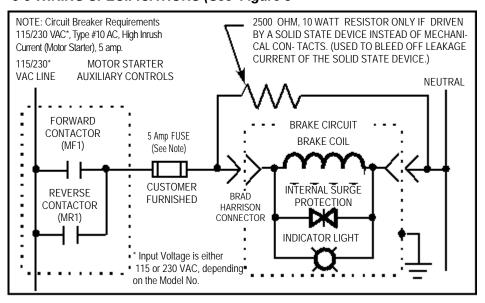
Figure 3 - Electrical Wiring Diagram
