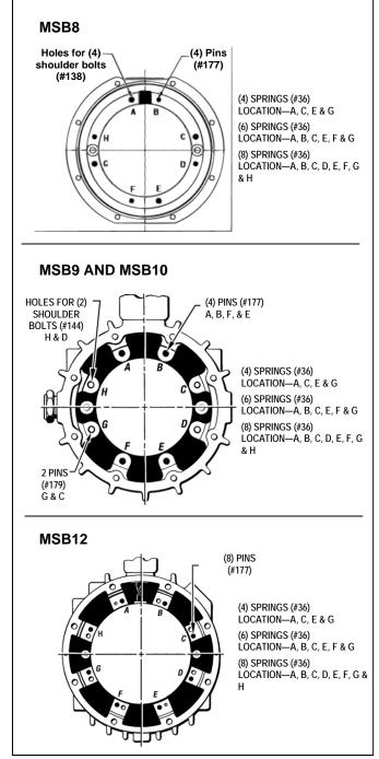
Figure 7.7—Correct placement of brake springs
