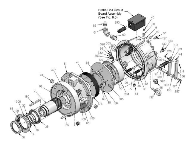
Figure 8.1.1 - Repair Parts - MSB8 MagnaShear Motor Brake
