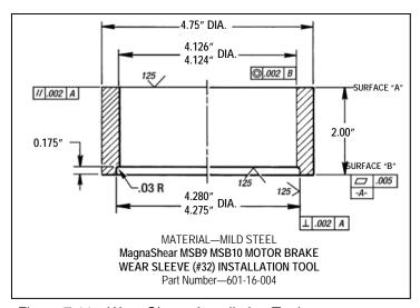
Figure 7.11—Wear Sleeve Installation Tool
