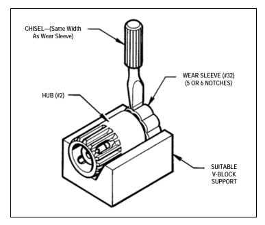
Figure 7.10—Removing Wear Sleeve (#32)
