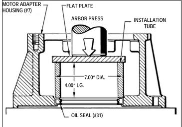
Figure 7.14 - Installing Oil Seal for MSB9 and MSB10
