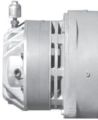
*Posistop* Motor Brakes are multiple surface, spring activated, pneumatic release braking devices that effectively dissipate the heat generated from electric motors requiring frequent starting and stopping,
