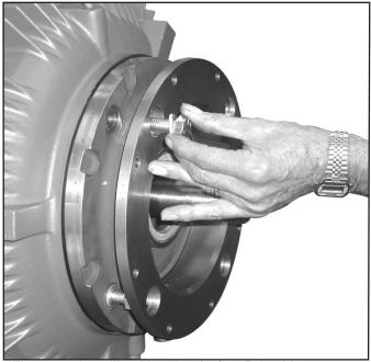
Figure 3 - Installing Housing (#8) to Drive Motor
