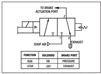
Figure 11 - Control Valve Schematic and Logic
