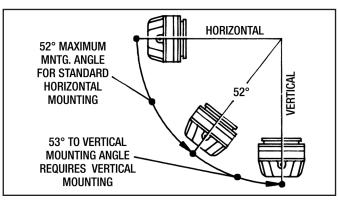
Figure 14 - Mounting Angle (Brake Down)
