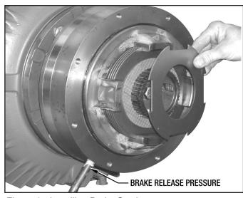
Figure 8 - Installing Brake Stack
