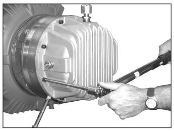
Figure 10 - Attaching End Housing
