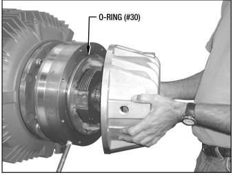
Figure 9 - Installing End Housing (#9)
