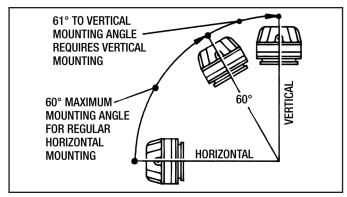
Figure 12 - Mounting Angle (Brake Up)
