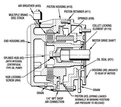
Figure 1 - Unit Description and Operation
