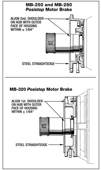
Figure 5 - Hub Alignment - Step 2
