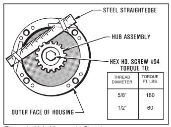
Figure 4 - Hub Alignment - Step 1
