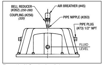
Figure 13 - Air Breather Installation
