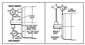
Figure 2 - Verifying Motor Specifications
