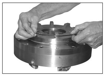
Figure 6 - Installing O-Ring (#33)
