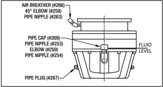
Figure 15 - Air Breather Installation (Brake Down)
