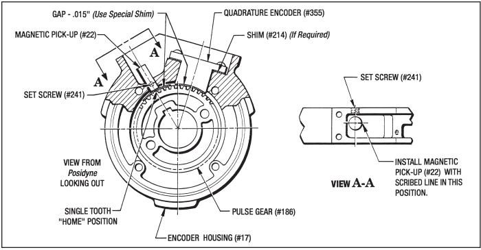
Figure 9.17 - Position Sensors Installation
