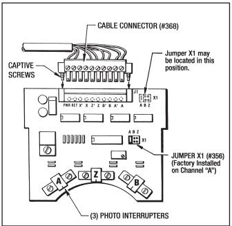
Figure 7.2 - Circuit Board Connector
