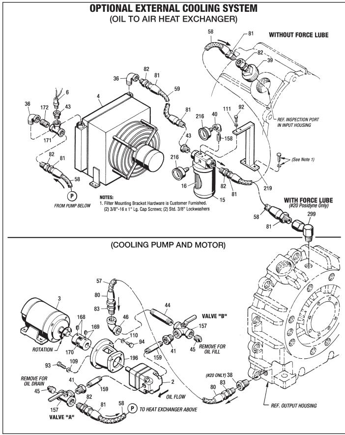
Figure 10.11 - External Cooling System
