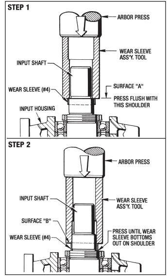
Figure 9.6 - Installing Wear Sleeve (#4) on #11 Posidyne
