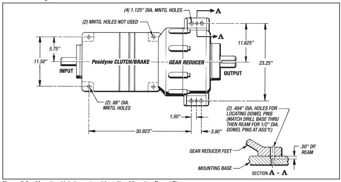
Figure 3.2 - Mounting Hole Layout and Installing Mounting Dowel Pins
