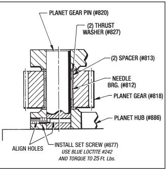
Figure 9.22 - Installing Planet Gears
