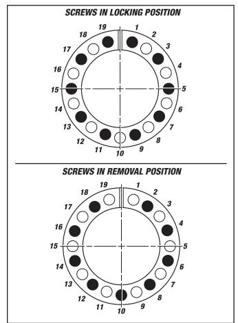
Figure 7.1 - Flywheel Locking Assembly Removal
