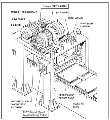
Figure 1.1 - Typical Single Revolution Application
