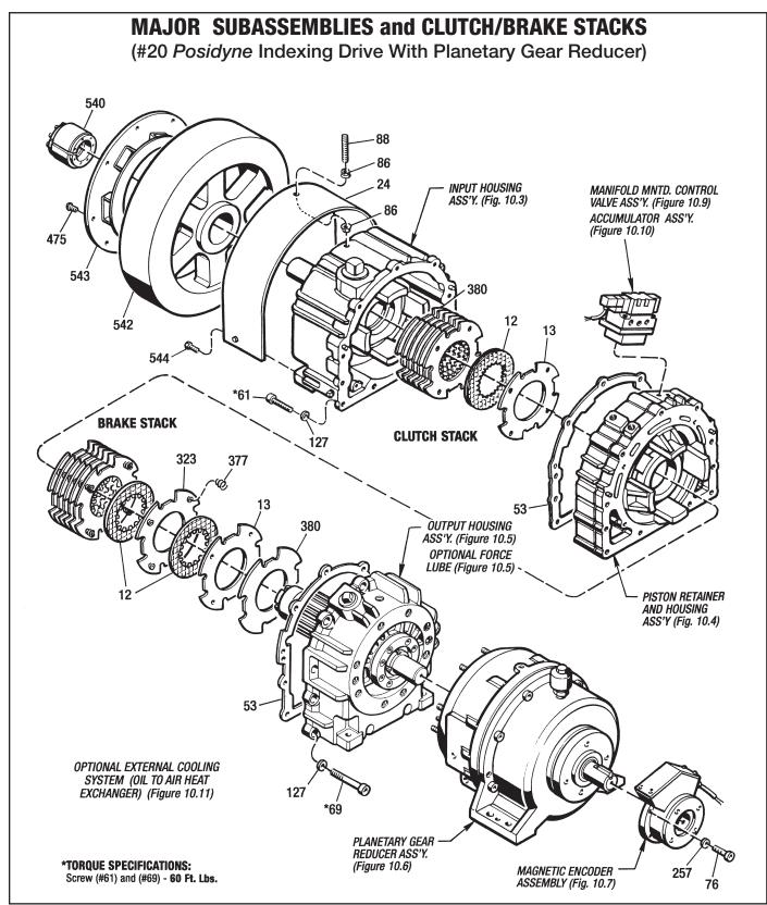
Figure 10.2 - #20 Posidyne Indexing Drive (With Planetary Gear Reducer)
