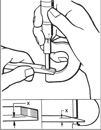
Figure 9.12 - Measuring Piston Stroke
