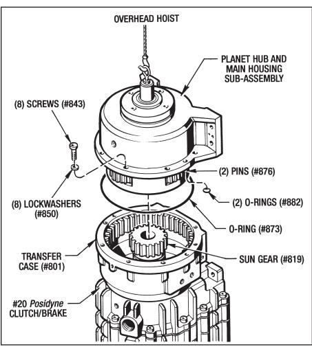
Figure 9.26 - Planetary Gear Reducer Installation
