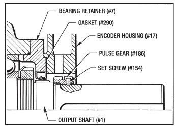
Figure 9.13 - Pulse Gear Alignment (#11 Posidyne)
