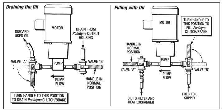
Figure 4.2 - Valve Positions for Draining and Filling Oil
