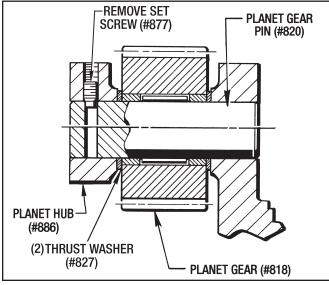
Figure 7.12 - Removing Planet Gear Pin (#820)
