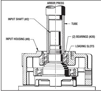
Figure 9.4 - Pressing Bearings (#26) into Input Housing
