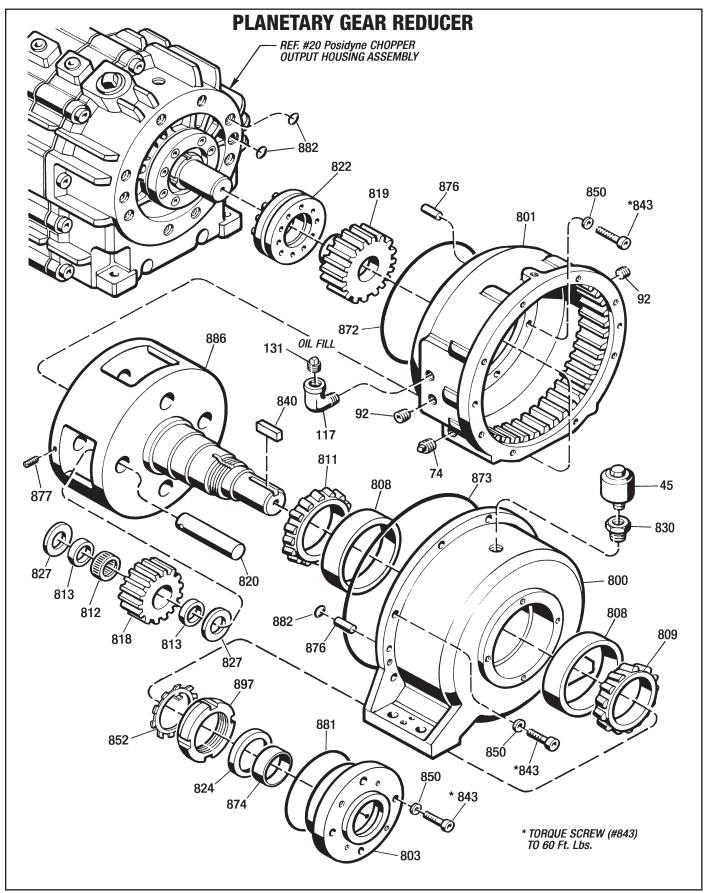
Figure 10.6 - Planetary Gear Reducer
