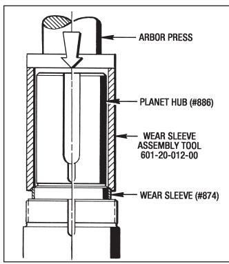
Figure 9.24 - Installing Wear Sleeve (#874)
