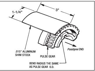
Figure 9.16 - Sensor Gap Shim
