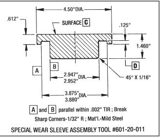
Figure 9.7 - Wear Sleeve Assembly Tool for #20 Posidyne
