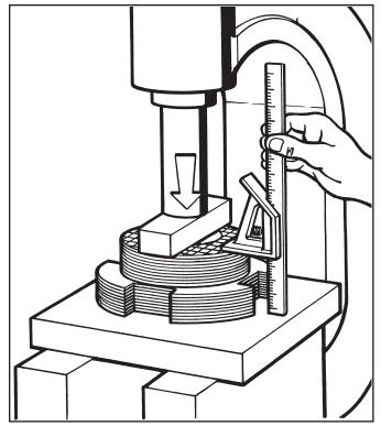
Figure 9.9 - Measuring Stack Height
