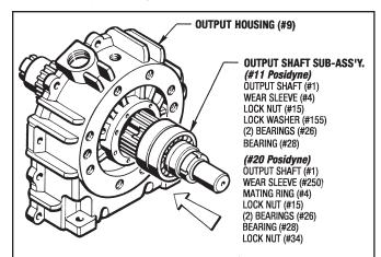
Figure 9.3 - Installing Output Shaft Sub-Assembly
