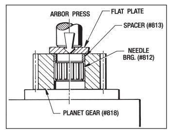
Figure 9.21 - Installing Needle Bearings (#812)
