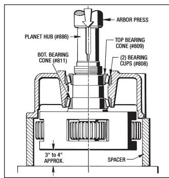
Figure 7.9 - Removing Planet Hub (#886)
