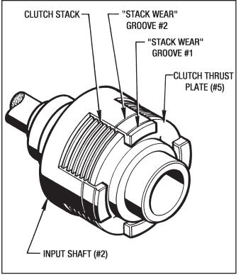
Figure 6.1 - "Stack Wear" Grooves
