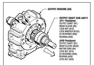
Figure 7.8 - Removing the Output Shaft
