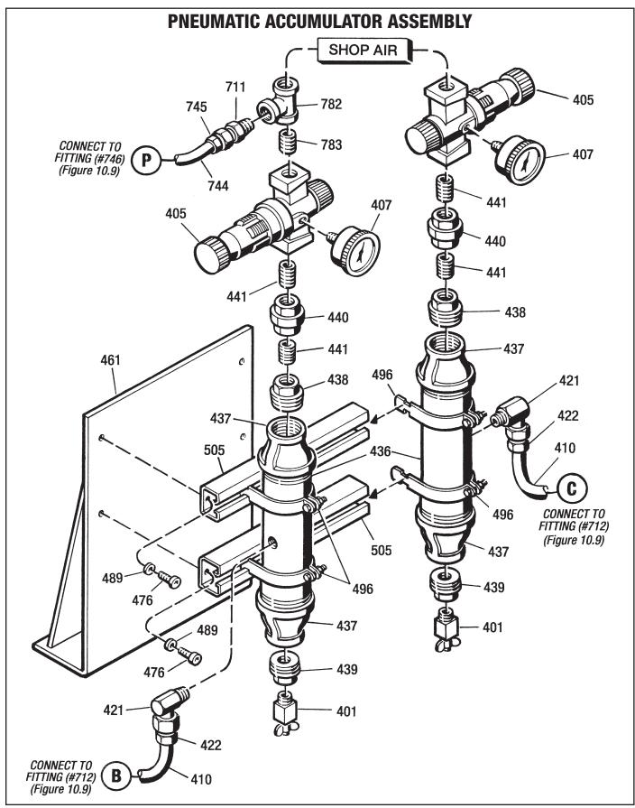
Figure 10.10 - Pneumatic Accumulator Assembly
