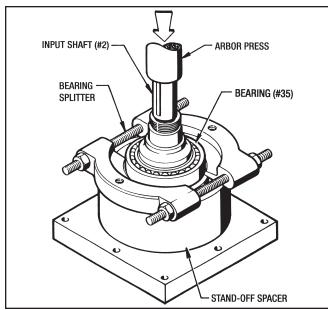
Figure 7.5 - Removing Bearing from the Input Shaft
