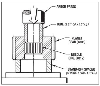
Figure 7.13 - Removing Needle Bearing (#812)
