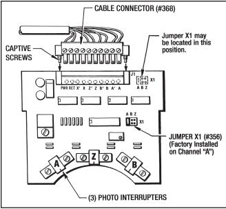
Figure 9.20 - Circuit Board Connector
