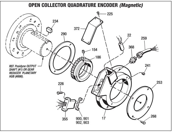
Figure 10.7 - Open Collector Quadrature Encoder (Magnetic)
