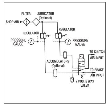
Figure 3.3 - Pneumatic Schematic
