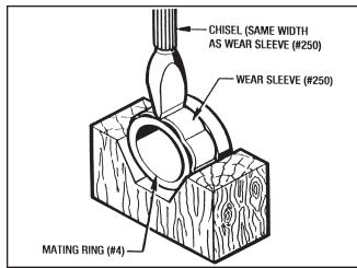
Figure 7.4 - Wear Sleeve Removal (#20 Posidyne Only)
