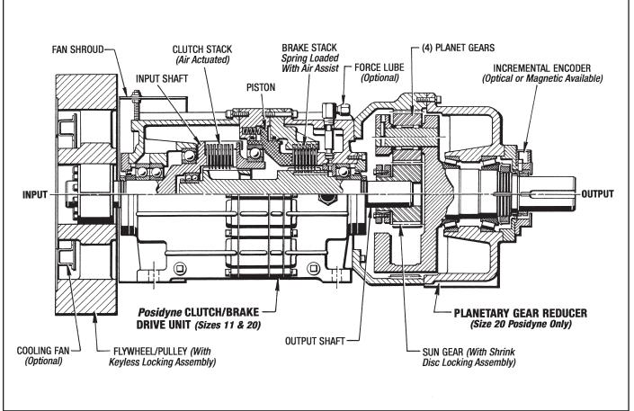
Figure 1.2 - Posidyne Indexing Clutch/Brake Drive
