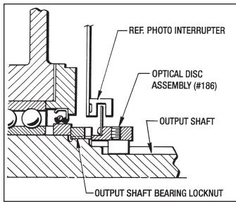
Figure 9.18 - Optical Disc and Hub Positioning
