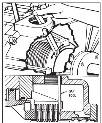
Figure 9.11 - Inserting Gap Tool
