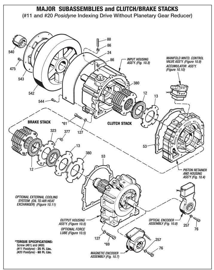
Figure 10.1 - #11 and #20 Posidyne Indexing Drive (Without Planetary Gear Reducer)
