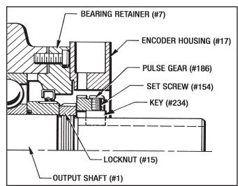
Figure 9.14 - Pulse Gear Alignment (#20 w/o Reducer)
