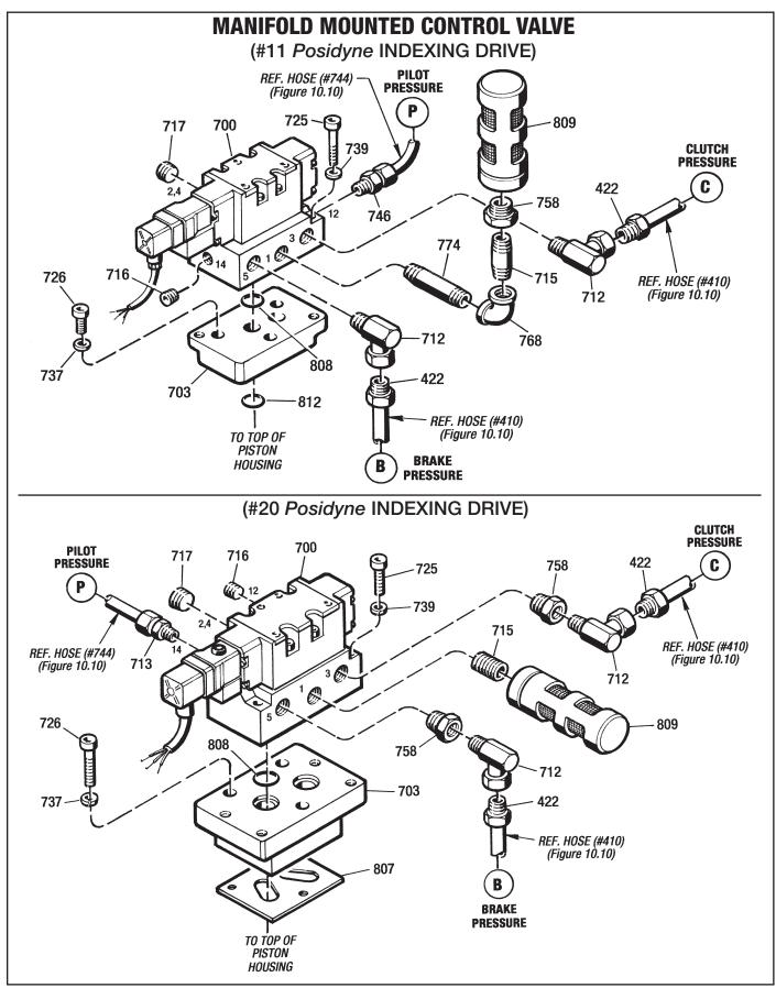
Figure 10.9 - Manifold Mounted Control Valve
