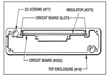
Figure 9.19 - Circuit Board Slots
