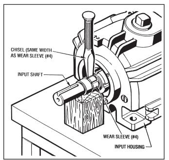
Figure 7.3 - Wear Sleeve Removal (#11 Posidyne Only)
