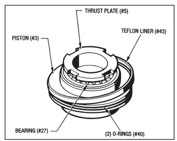
Figure 7.6 - Piston Sub-Assembly
