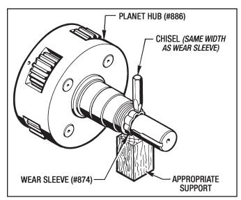
Figure 7.11 - Removing Wear Sleeve (#874)
