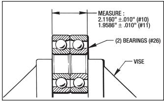
Figure 9.1 - Measuring Thickness of Bearings (#26)
