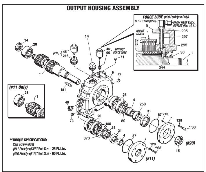
Figure 10.5 - Output Housing Assembly
