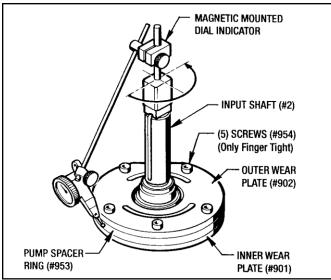
Figure 9.07 - Checking Concentric Alignment
