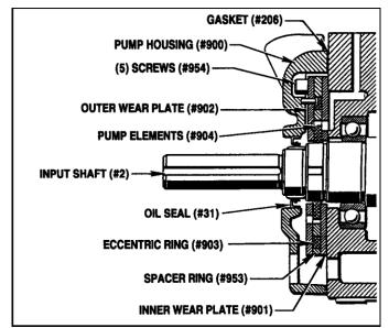
Figure 7.02 - Pump Disassembly
