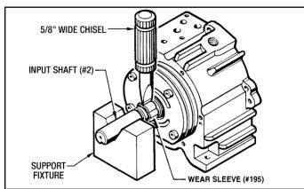
Figure 7.03 - Removing Wear Sleeve (#195)
