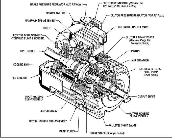
Figure 1.1 - EL-02 Posidyne Clutch/Brake Description
