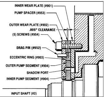
Figure 9.06 - Hydraulic Pump Assembly (Cross Section)
