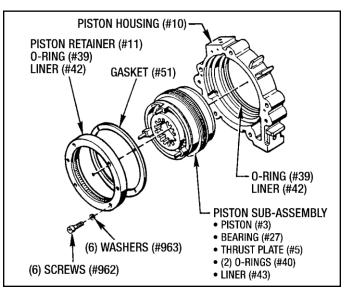
Figure 7.06 - Removing Piston From Piston Housing
