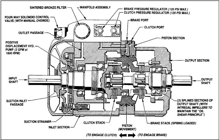
Figure 1.03 - EL-02 Posidyne Clutch/Brake Operation
