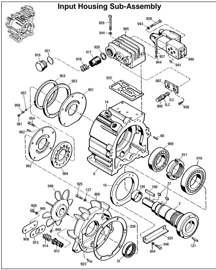
Figure 10.02 - Input Housing Sub-Assembly
