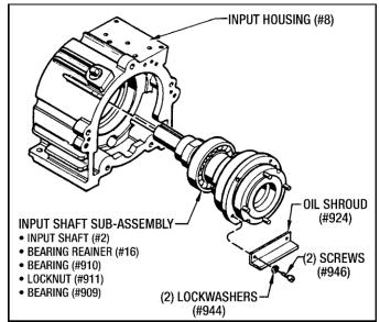
Figure 9.04 - Installing Input Shaft Into Input Housing
