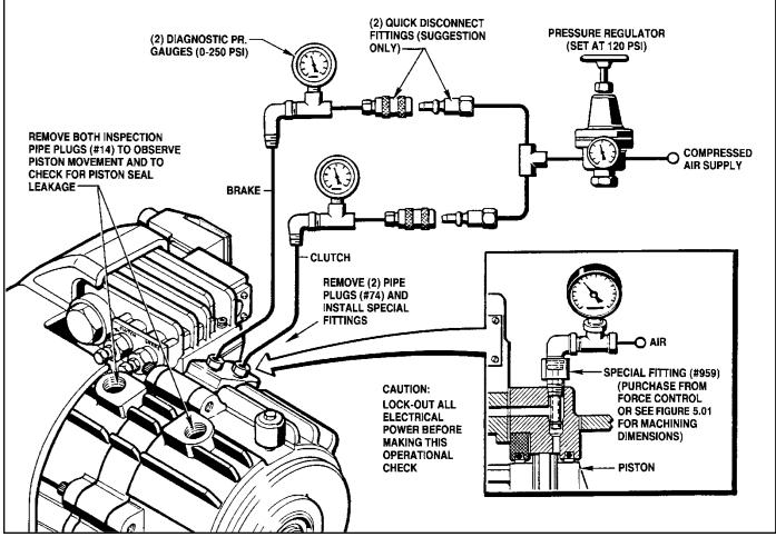
Figure 5.02 - Pneumatic Set-Up For Operations Check
