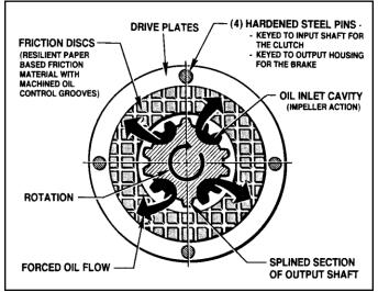
Figure 1.02 - The "Oil Shear" Principle
