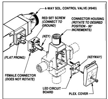
Figure 3.02 - Electrical Connector
