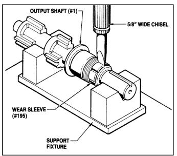
Figure 7.09 - Removing Wear Sleeve From Output shaft
