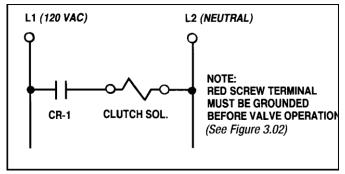
Figure 3.01 - Electrical Wiring Diagram
