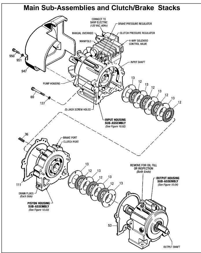
Figure 10.01 - Main Sub-Assemblies & Clutch/Brake Stacks
