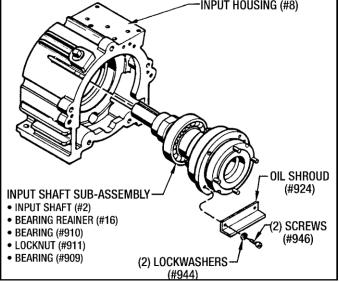
Figure 7.04 - Removing The Input Shaft
