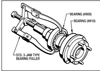
Figure 7.05 - Removing Bearing (#909)
