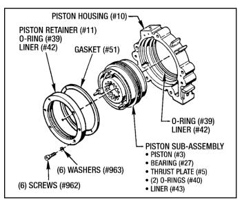
Figure 9.03 - Piston Housing Sub-Assembly
