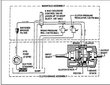
Energizing the control valve directs the oil to the R.H. side of the piston, forcing it to the left clamping the Clutch Stack. Driving torque is then transmitted from the input shaft, utilizing the "*Oil Shear Principle*", to the output shaft.
