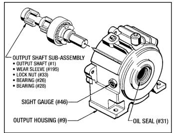
Figure 9.01 - Output Housing Reassembly
