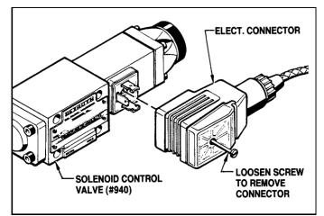
Figure 7.01 - Disconnecting The Electrical connector
