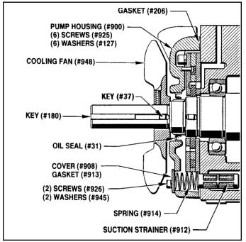
Figure 9.08 - Pump Housing, Suction Strainer & Cooling Fan
