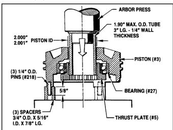
Figure 7.07 - Removing Bearing (#27)
