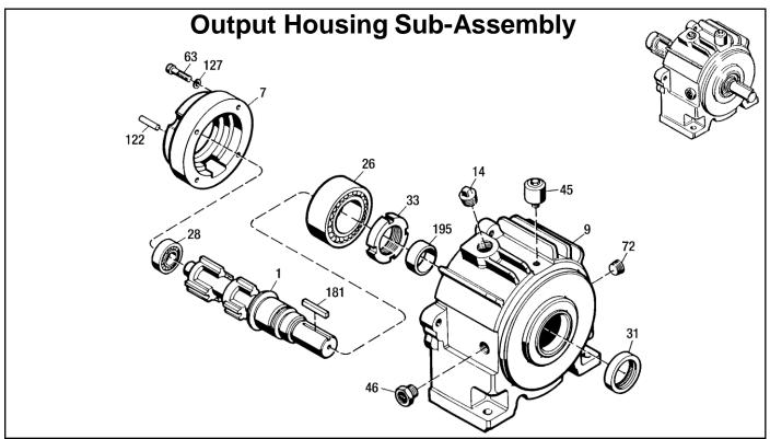
Figure 10.04 - Output Housing Sub-Assembly
