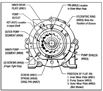
Figure 9.05 - Hydraulic Pump Assembly (End View)
