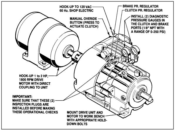
Figure 5.03 - Hydraulic Operational Checks
