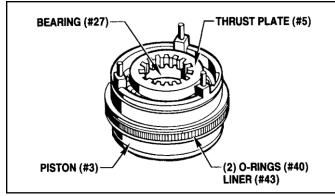
Figure 9.02 - Piston Sub-Assembly
