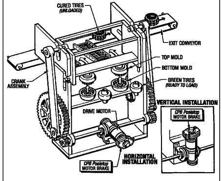
Figure 1.1 - Tire Curing Press
