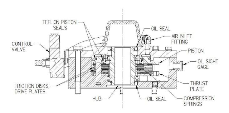
Figure 1.2 - Curing Press Brake Section
