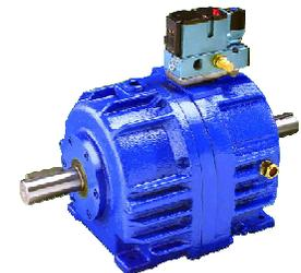
**Fan Cooling Enables Higher Radiation Cooling** —By adding fan cooling to the unit the housing is continuously cooled enabling greater cooling to the fluid ( as much as 4.5 times non fan cooling). Fan cooling works on applications when the input shaft rotates at high speed (1800 or 1200 RPM). At low speed there is not enough air flow to do much good. In addition the surrounding air temperature will affect the amount of cooling.
