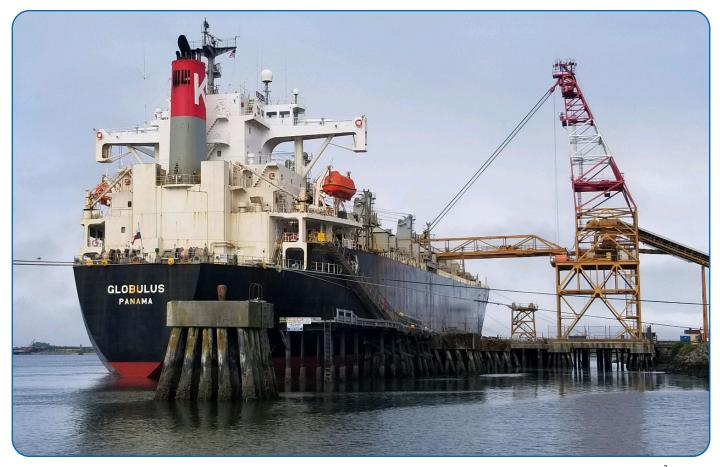
with a telescopic pneumatic pipe that can extend, retract, and rotate a full 360 degrees to allow the longshoremen to distribute chips evenly in the vessel holds. This loading head uses a Force Control MagnaShear MSB6 motor brake coupled to a 15 HP motor to start and stop the position of the loading head to optimize the vessel loading process.
