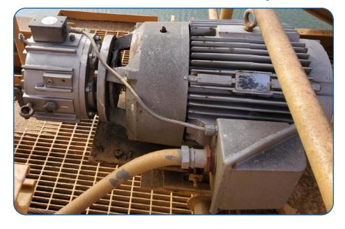
In addition to transmitting torque, a patented fluid recirculation system helps to dissipate heat which causes friction disc wear and eventual failure in traditional dry brakes. Along with heat removal and torque transmission, the fluid serves to continually lubricate all components of the oil shear brake, increasing their service life.
