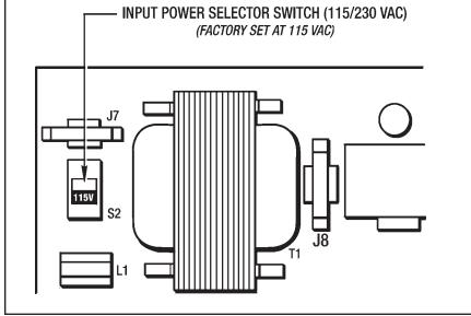
Figure 2.4 - Input Power Selector Switch
