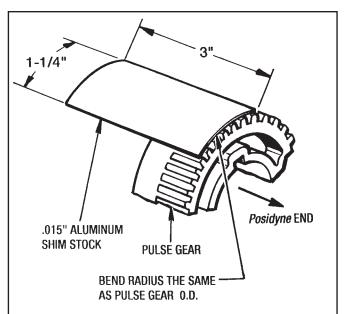
Figure 6.5 - Sensor Gap Shim
