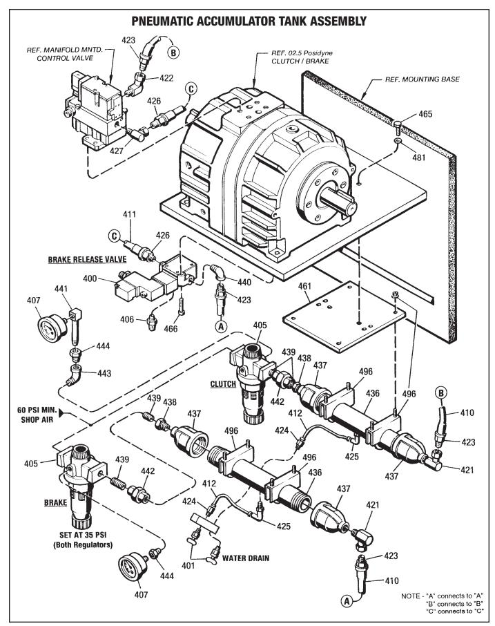
Figure 7.2 - Pneumatic Accumulator Tank Assembly FORCE CONTROL INDUSTRIES, INC.
