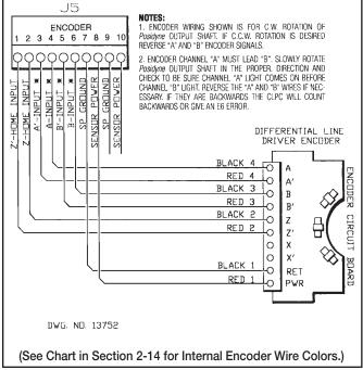
Figure 2.10 - Wiring Diagram - Terminal Block J5 (Differential Line Driver Encoder with Internal Home Sensor)
