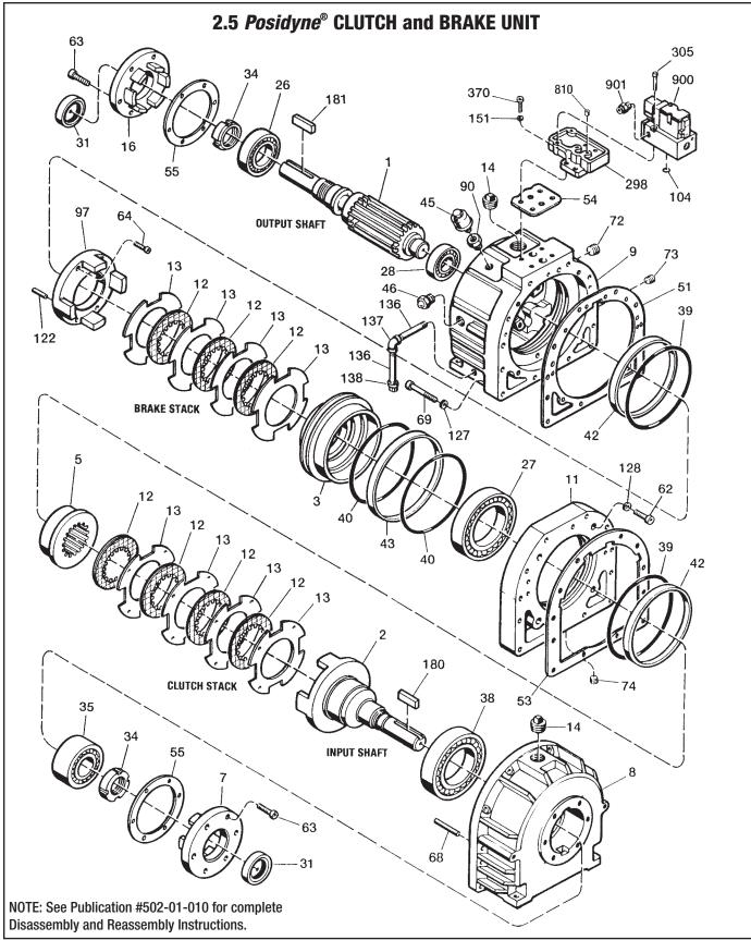
Figure 7.7 - 2.5 Posidyne Clutch/Brake Unit
