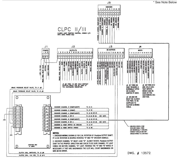
Figure 2.13 - Wiring Diagram - Junction Box to CLPC Control (With Differential Line Driver Encoder)
