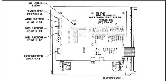
Figure 3.4 - CPU Board Component Location
