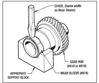
Figure 6.12 - Removing Wear Sleeve (#874)
