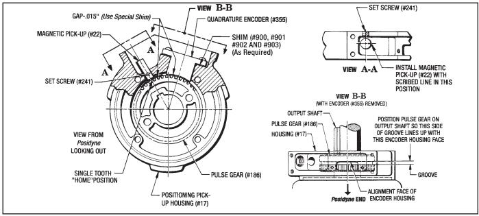
Figure 6.6 - Position Sensors Installation
