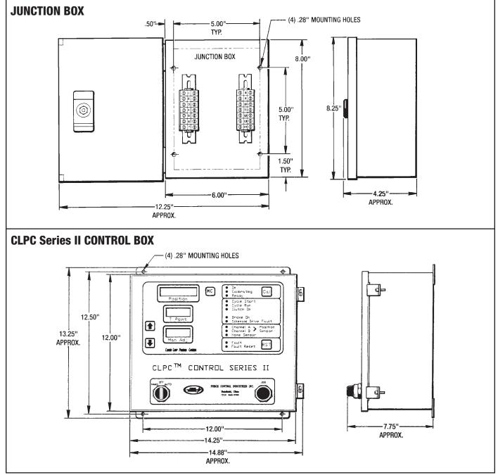
Figure 2.3 - CLPC Control and Junction Box Dimensions
