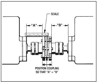
Figure 6.11 - Coupling Alignment
