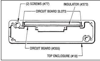
Figure 6.9 - Circuit Board Slots
