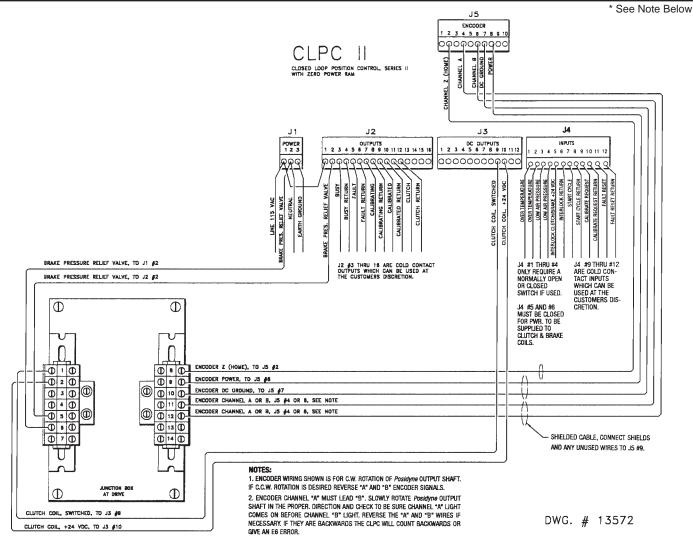
Figure 2.11 - Wiring Diagram - Junction Box to CLPC Control
