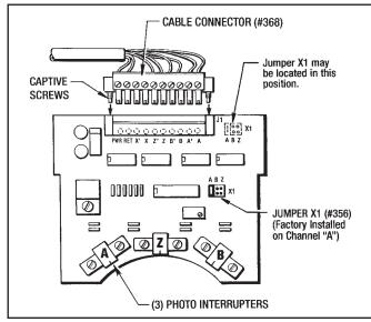
Figure 6.7 - Circuit Board Connector
