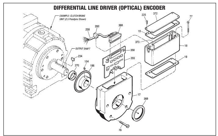
Figure 7.4 - Differential Line Driver (Optical) Encoder
