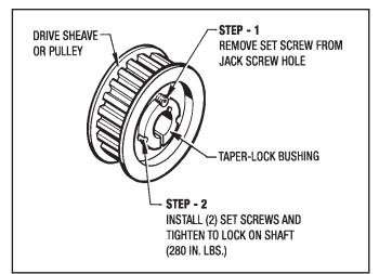
Figure 6.2 - Installation of Drive Sheaves
