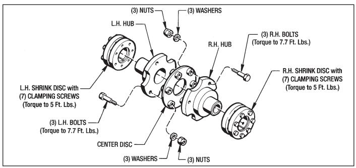
Figure 6.10 - Drive Coupling Elements
