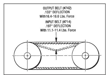
Figure 6.4 - Drive Belt Tensioning
