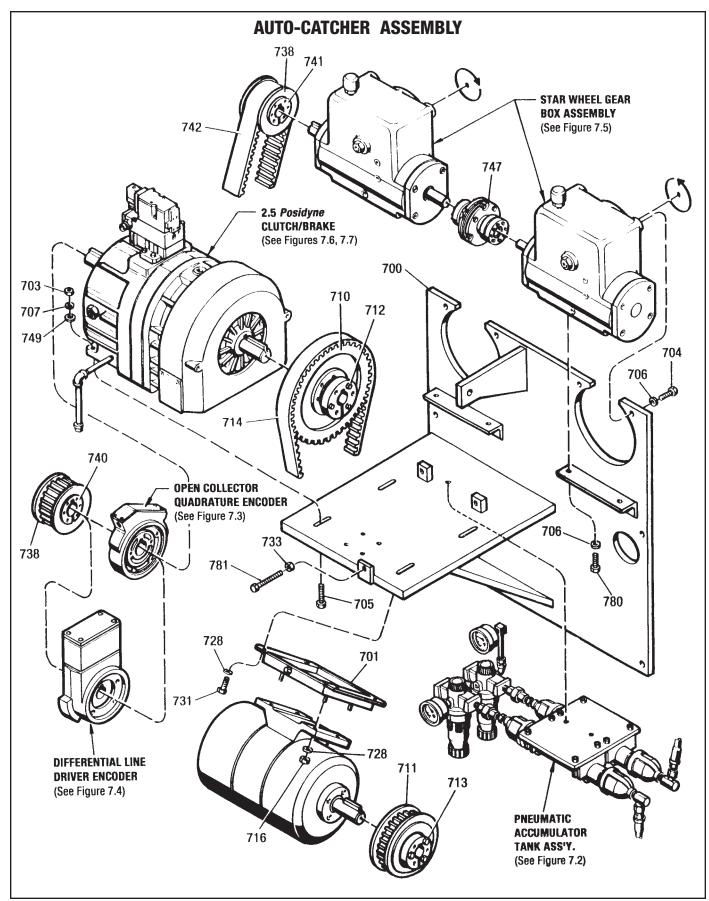
Figure 7.1 - Auto Catcher Assembly FORCE CONTROL INDUSTRIES, INC.
