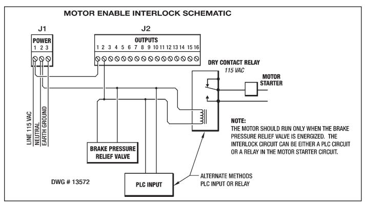
Figure 2.5 - Motor Interlock Schematic
