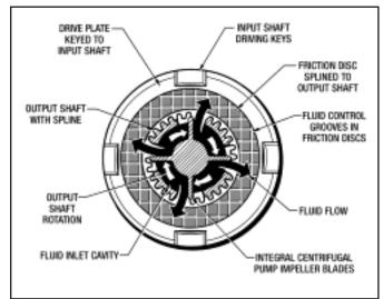
Figure 1.2 - The Oil Shear System
