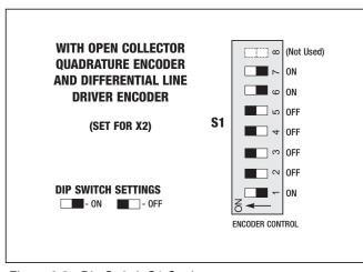
Figure 3.2 - Dip Switch S1 Setting
