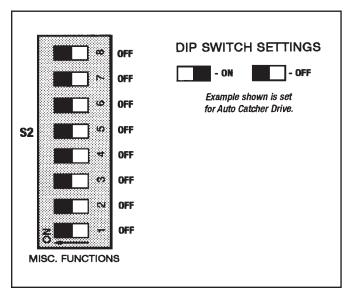
Figure 3.7 - Setting Misc. Functions (Dip Switch #S2)
