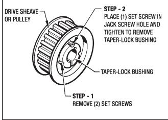
Figure 6.1 - Removal of Drive Sheaves
