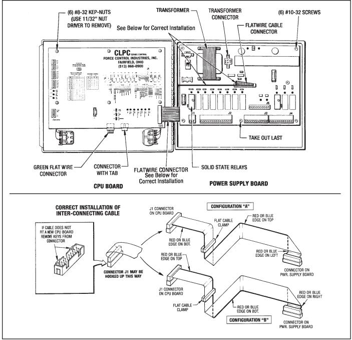
Figure 6.14 - Replacing Circuit Boards
