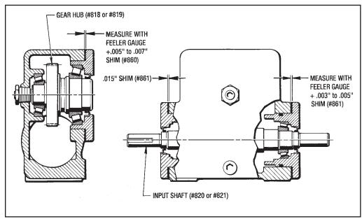
Figure 6.13 - Determining Shim Thickness of Bearing Retainers
