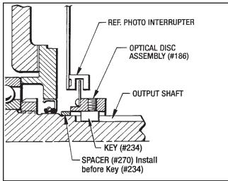
Figure 6.8 - Optical Disc and Hub Positioning
