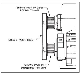
Figure 6.3 - Sheave Alignment
