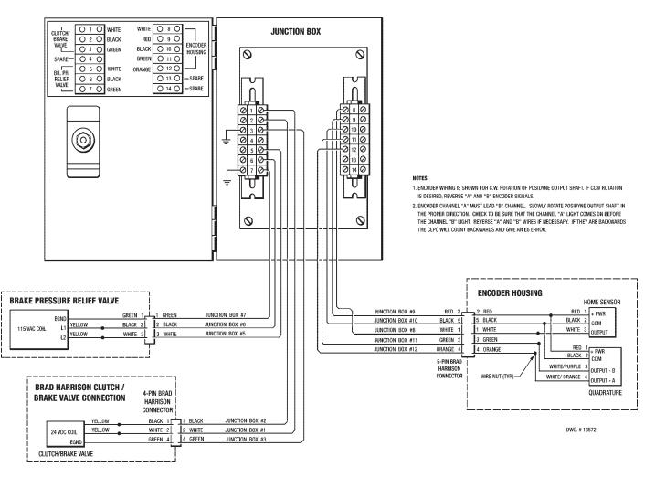
Figure 2.12 - Wiring Diagram - Junction Box to Actuation Valves and Position Encoder (Open Collector Quadrature Encoder)
