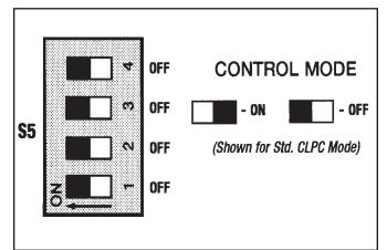
Figure 3.6 - Setting Dip Switch S5 (Control Mode)
