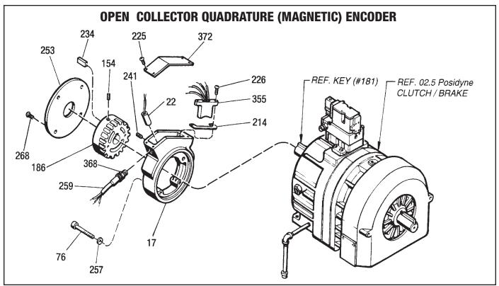
Figure 7.3 - Open Collector Quadrature (Magnetic) Encoder
