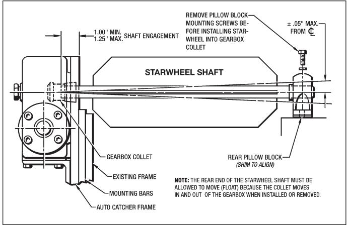
Figure 2.1 - Drive Unit Installation
