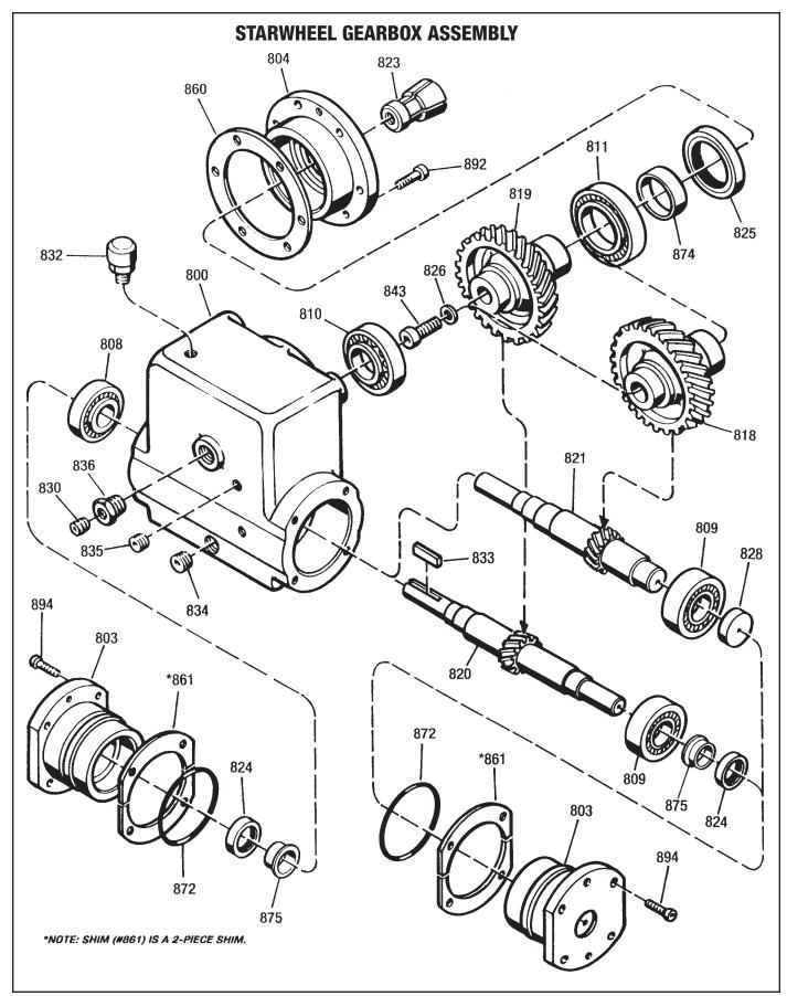
Figure 7.5 - Starwheel Gearbox Assembly FORCE CONTROL INDUSTRIES, INC.
