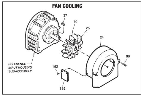
Figure 7.6 - Fan Cooling
