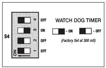
Figure 3.5 - Watch Dog Timer Dip Switch S4
