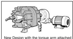
New Design with the torque arm attached to the *Positorq* Clutch input shaft.
