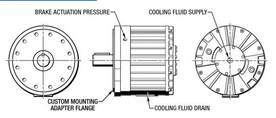
These **Flange Mounted Positorq Brakes** normally require special modifications to fit a specific application. Consult our factory for certified installation, dimensional drawings and assistance in ordering.
