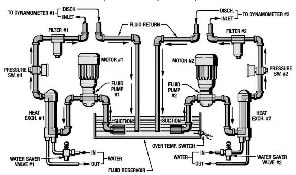
NOTE: Kidney Filtration can also be included on this Dual-Pump Forced Lube Cooling System.
