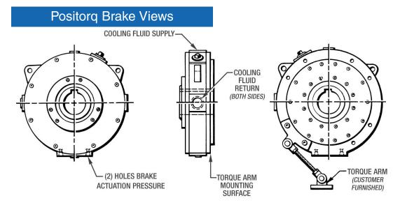
These **Shaft Mounted** *Positorq* **Brakes** normally require special modifications to fit a specific application. Consult our factory for certified installation, dimensional drawings and assistance in ordering.
