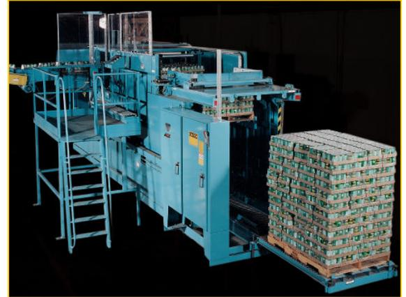
**Yes, Palletizers and they are critical to their operations.** Whether they are bottling Coke or Pepsi, Budweiser or Miller, a critical machine in a bottling plant is the High Speed Palletizer. These high speed palletizers are the last step before product can be shipped to distribution facilities or stores. They are packing 400 12-pack cases on a skid in approximately 2 minutes. The total skid can weigh as much as 4000 lbs.
