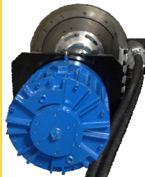
TB-20 Positorq Load Brake used to test a hydraulically operated large engine starter motor. Testing was designed for 24 hr continuous testing.
